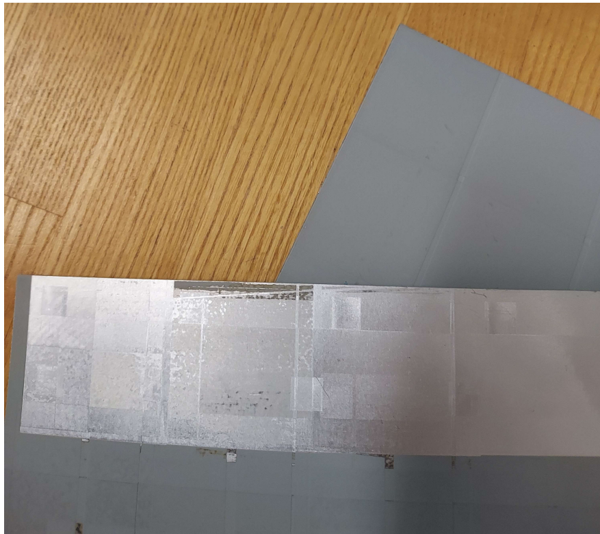
Figure 7.3: Contrast of paint layers on two coupons: single versus multiple passes.
