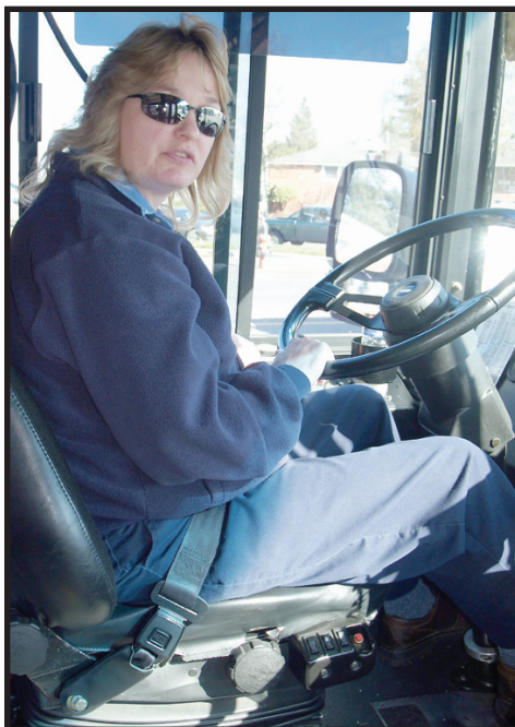
Adjustable seats with shock absorbers and hydraulics help ease back pain of TriMet bus operator and ATU member Sandy Guengerich.
