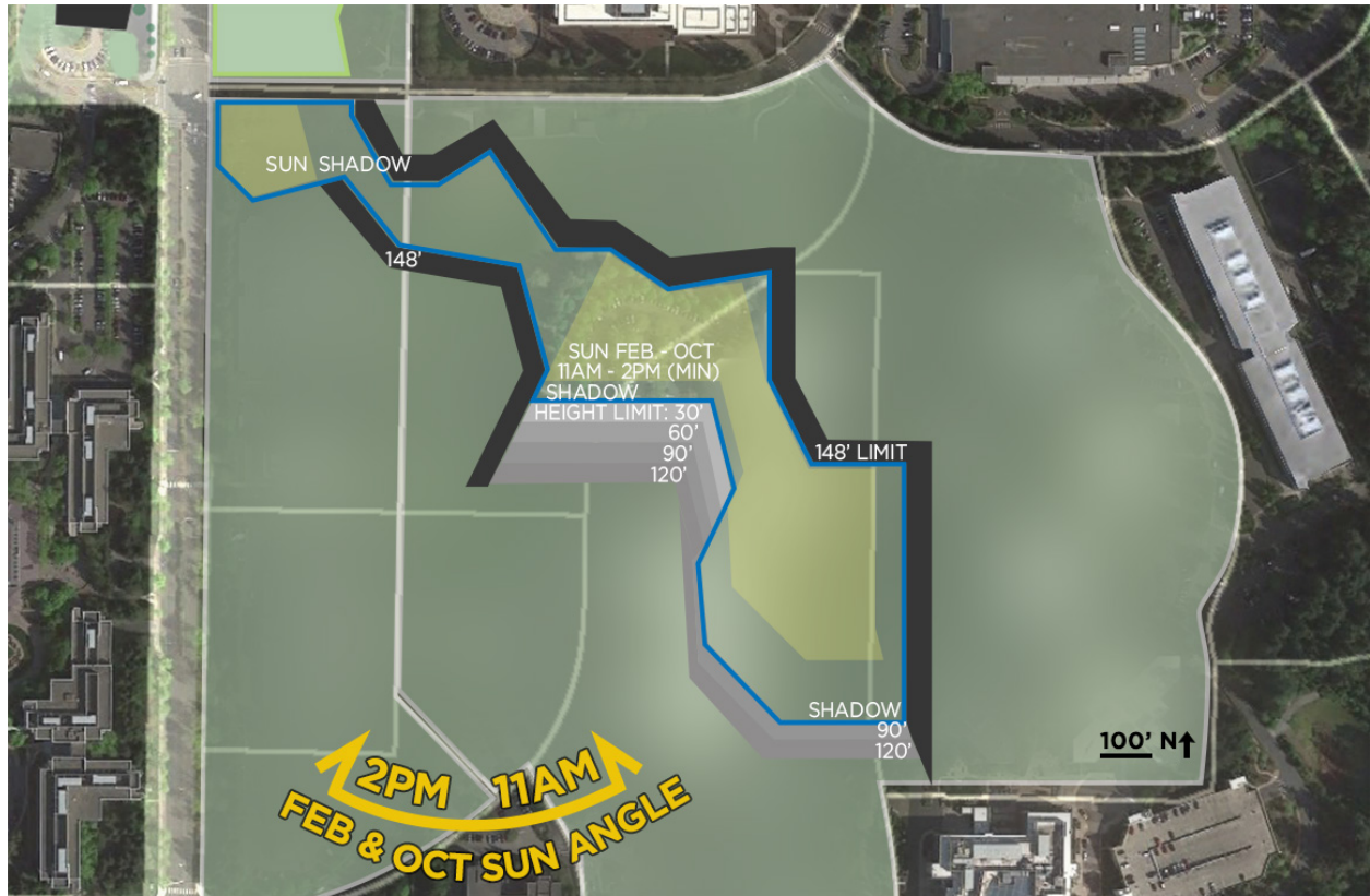
Figure 43. Proposed axial network of plazas (blue) with overlaid results of building mass and shadow study. The sunny area (yellow) will have direct sunlight from, at a minimum, 11 AM to 2PM from February through October. The height limited areas (greys) are an opportunity to create an employees-only second or third floor outdoor space. By Author.
