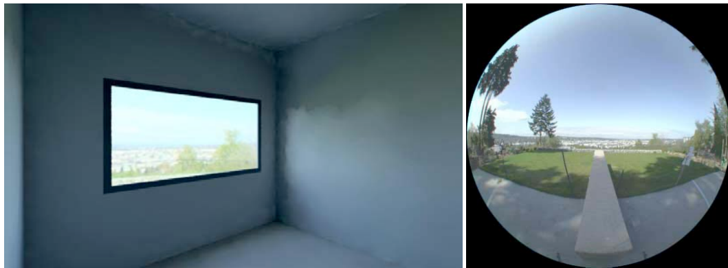
Figure 4.09: An interior view of a room with a single window (left) can be lit using a vertical light probe (right) and a customized translation equation.
