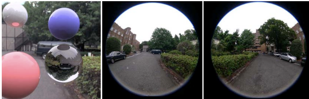
Figure 4.22: A model with a camera viewpoint (left) that avoids showing the seam between the two light probes (center and right) used to illuminate it [29].
