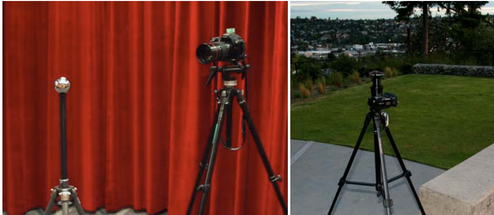
Figure 4.02: Different setups needed for HDR image capture – 360° capture (left) [35] and 180° capture (right).
