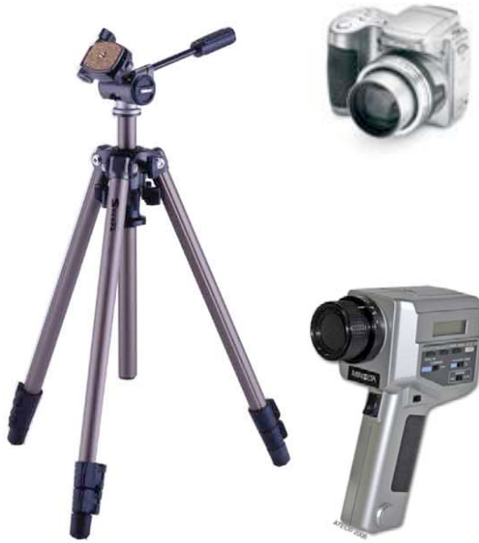
Figure 2.05: Basic equipment needed to capture an HDR photograph: a tripod, digital camera, and luminance meter.
