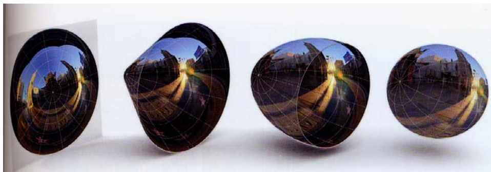
Figure 3.07: Use of environment mapping to translate a 2D image of a 360° environment into a 3D spherical object [18].
