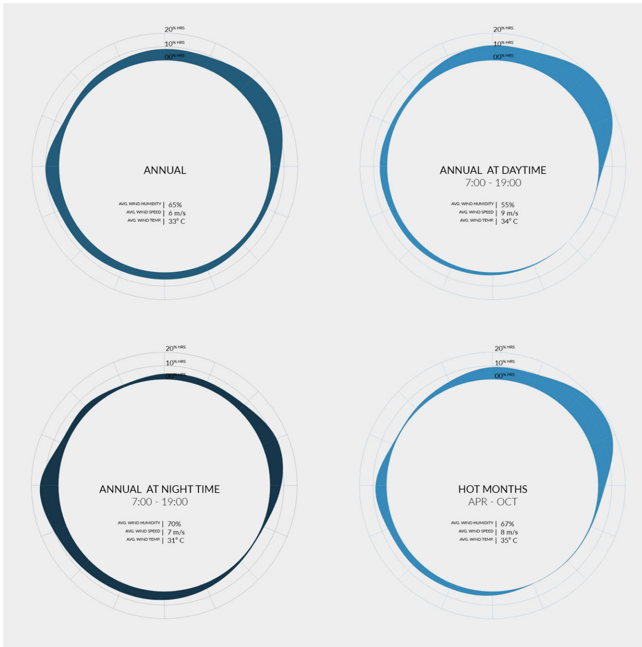
fig 4.08 | Climate data from Muscat International Airport collected from 2003 - 2017, representing prevailing wind direction at different time periods specified by Month and hours.
