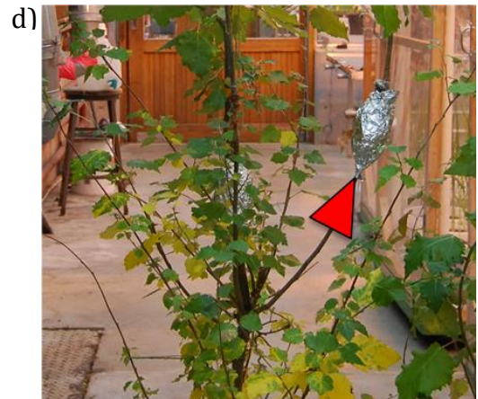
Fig 5. Sap flow sensor method. a) Diagram of miniature external sap flow gauges for capturing plant water movement (John et al. 2020, in prep. ). b) Upside down view of one of the sapflow gauges – temperature probes and heater are visible. c) Sensor installed on a poplar tree branch. Sensors were covered with plastic for thermal isolation and water protection. d) Location where sensors were installed – directly below each canopy soil system (red arrow corresponds to sensor).
