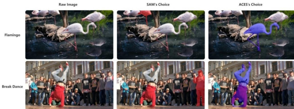
Figure 6.2. Representative candidate-selection improvements in multi-instance scenes: raw images (left), SAM confidence-based selections (middle), and ACES selections (right) for the flamingo and breakdance sequences.
