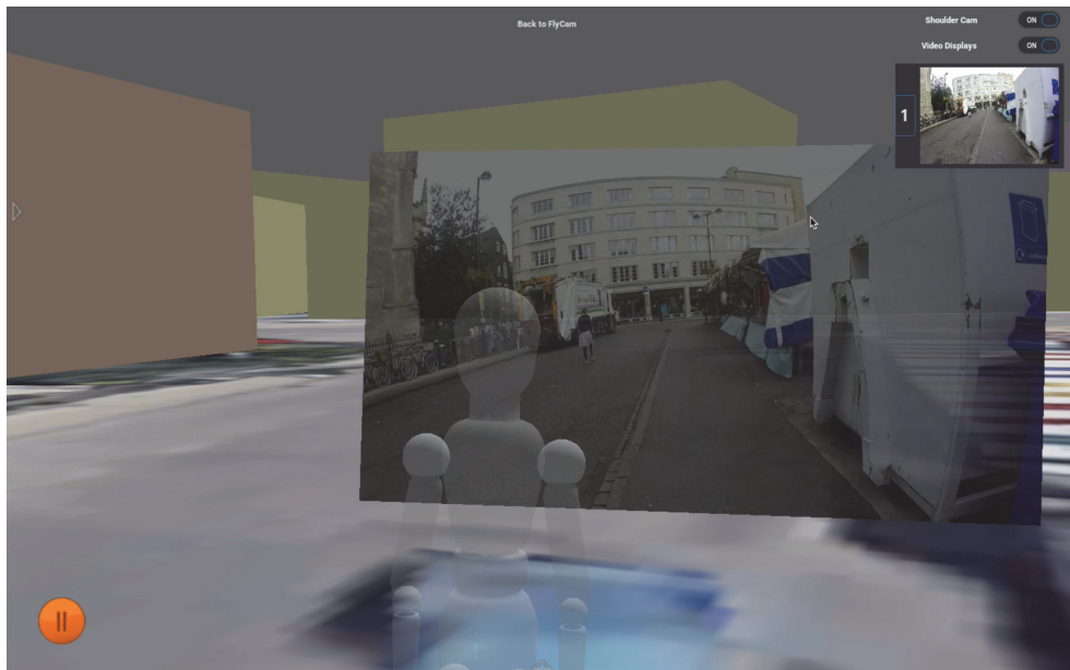
Fig. 2. ForensicMesh: the image shows a parsimoniously rendered citiscape, with only coloured outlines of surrounding buildings. Within the scene, a video plays on a suspended frame, with a human figure in front of it representing the viewpoint of the police officer whose body-worn camera originally captured this video.
