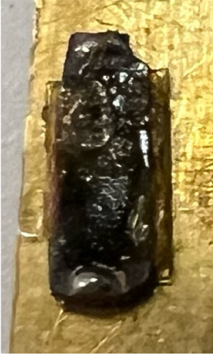
Figure A.5: Image of the carbon composition sensor as the resistance temperature sensor.
