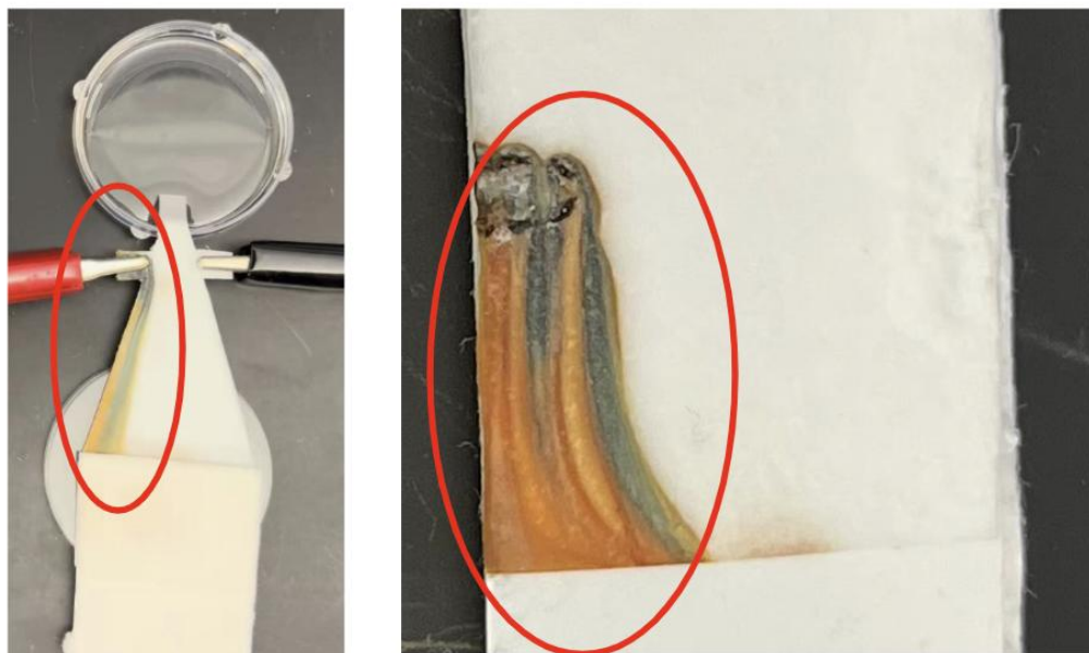
Figure 29: Colored streaks suggesting corrosion downstream of the alligator clip electrode.
