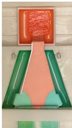
Appendix 1 Figure 6: A picture of the flow test with color dye on the geometry shown in Appendix 1 Figure 5.
