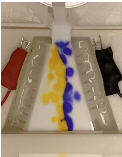
Figure 21: An image showing pH shift after a run with initial pH at the three buffer inlets were set to be pH 6.5, 7.0, 8.0 (running buffer: 100 mM ACES + 500 mM NaCl), indicated by the color change of BPB.
