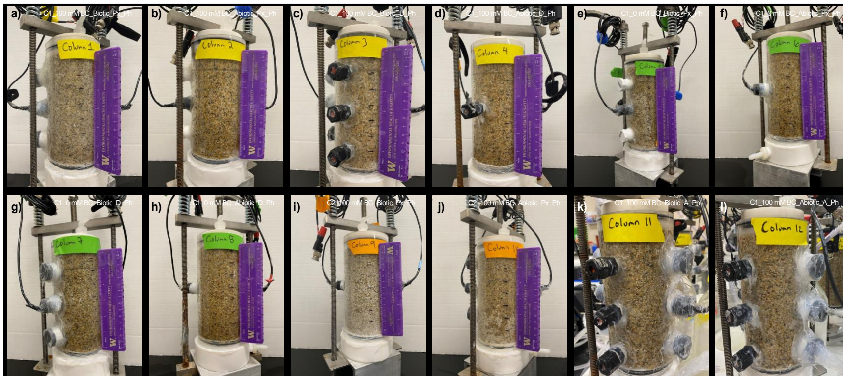
Figure 3.22. Images of the final conditions for all citrate oxidation columns. Images are presented for columns: (a) C1_100 mM BC_Biotic_Px_Ph, (b) C1_100 mM BC_Abiotic_Px_Ph, (c) C1_100 mM BC_Biotic_D_Ph, (d) C1_100 mM BC_Abiotic_D_Ph, (e) C1_0 mM BC_Biotic_Px_Ph, (f) C1_0 mM BC_Abiotic_Px_Ph, (g) C1_0 mM BC_Biotic_Px_Ph, (h) C1_0 mM BC_Abiotic_Px_Ph, (i) C2_100 mM BC_Biotic_Px_Ph, (j) C2_100 mM BC_Abiotic_Px_Ph, (k) C1_100 mM BC_Biotic_A_Ph, and (l) C1_100 mM BC_Abiotic_A_Ph
