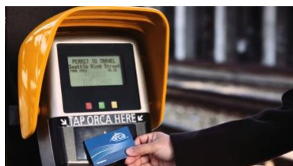
Figure 5. Sensor for "tapping" ORCA cards on entering and exiting light rail stations
