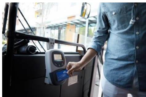
Figure 6. Sensor for "tapping" ORCA cards on entering the bus
