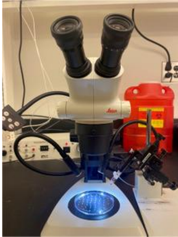
Figure 4.1.3. Microinjection rig setup with loaded capillary and tadpoles oriented for injection
