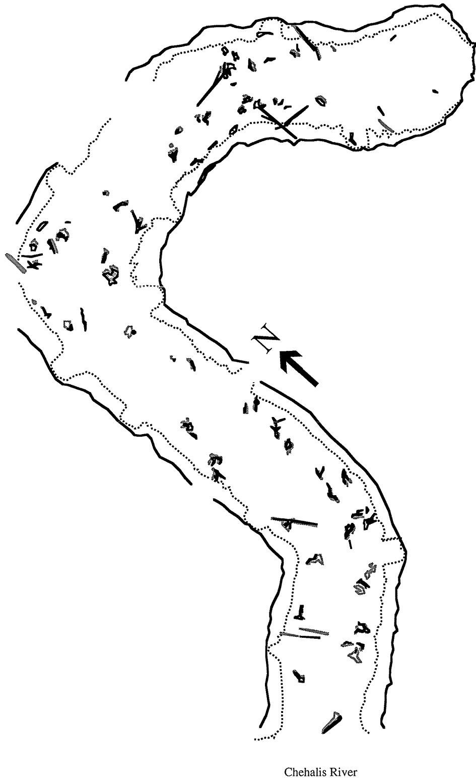
FIGURE 11.—Overlap in large organic debris (LOD) between 1993 (heavy black lines) and 1995 (light gray lines) in created slough in brackish region of upper Chehalis River estuary, Grays Harbor, Washington. The 1995 lines overlay the 1993 to best illustrate the general decrease in LOD area, which is likely due to sedimentation or settling. The solid black line (perimeter) is the edge of upland (excavated area of slough) and the dashed line is the lower edge of the Carex lyngbyei sedge distribution. Lines are discontinuous where aerial photo coverage was incomplete.
