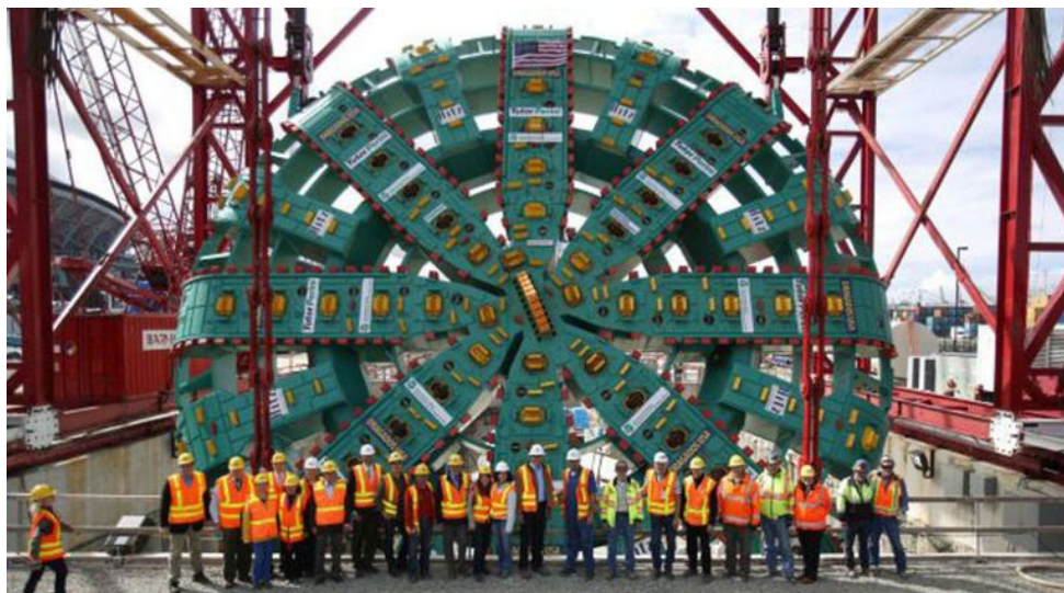
Figure 42 "Bertha", the largest tunnel boring machine in the world used to dig the SR-99 tunnel
