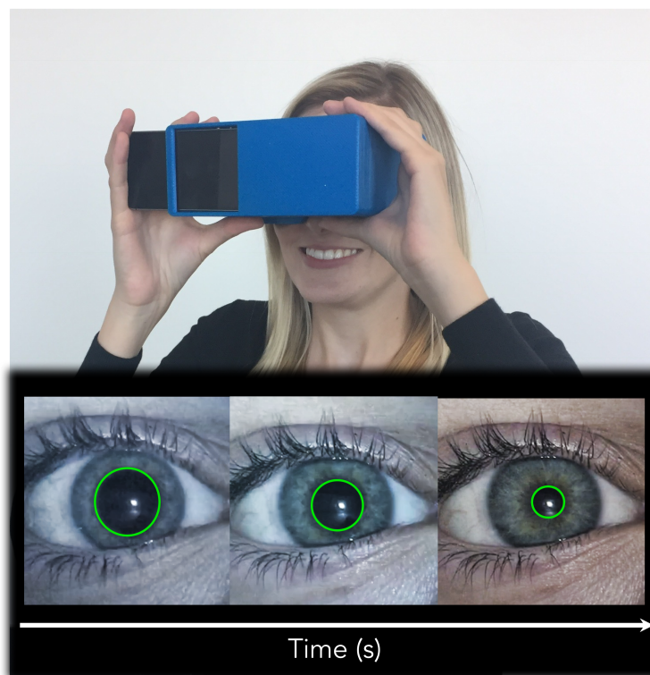
Figure 5.1: PupilScreen is a system that measures the pupillary light reflex to determine the severity of a traumatic brain injury. A smartphone app records a video of the patient's eyes as the camera's flash illuminates them. The VR headset-like box controls the position of the phone and the lighting that reaches the eyes.
