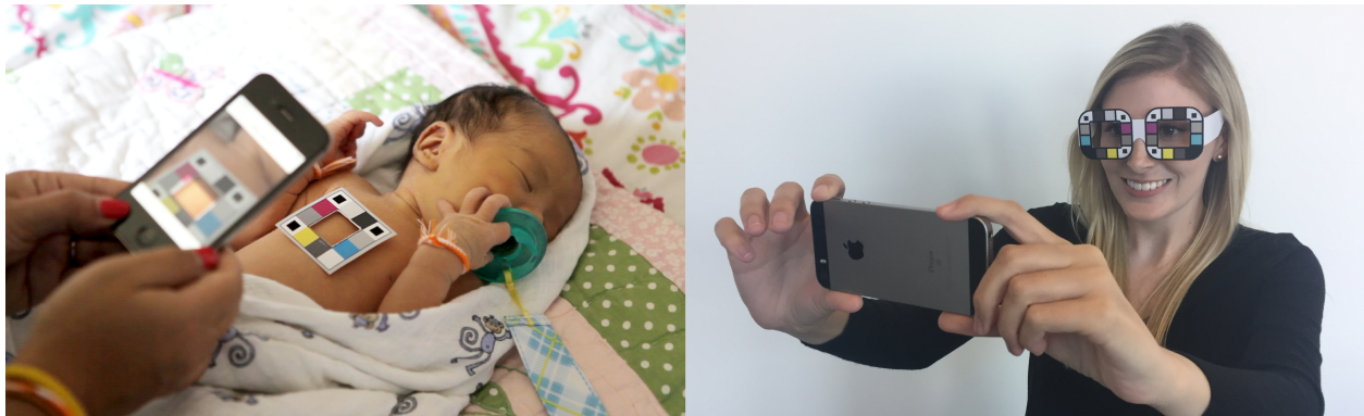
Figure 6.1: To account for different lighting conditions and camera sensors, both (left) BiliCam and (right) BiliScreen incorporate paper accessories with colored squares that can be used as calibration references.
