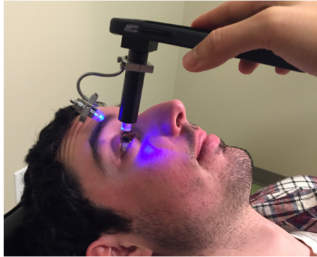
Figure 3.1: The proposed system emulates fixed-force applanation tonometry using the hardware adapter pictured above. The clear acrylic cylinder is allowed to move freely within the black casing pictured so that its mass provides a constant force on the patient's eye.
