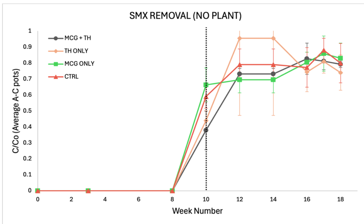
Figure 4.10: Sulfamethoxazole removal efficiency over time in pots with no plants amended with either TH@MCG , TH only, MCG only, or no amendment (soil control). *Line at week 10 indicates contaminant concentration increase because there was complete contaminant removal prior ( C/C_0 = 0 ).
