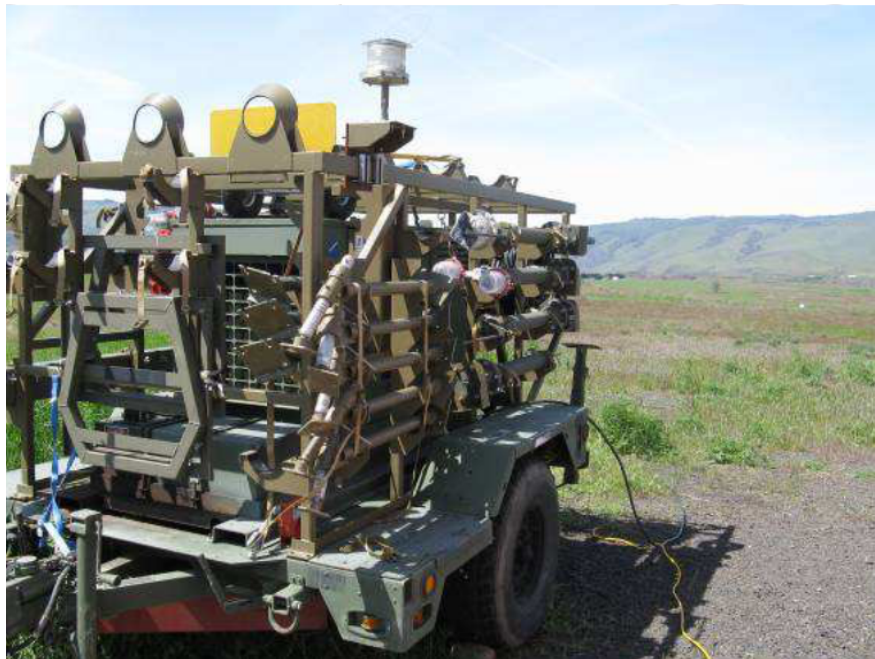
Figure 3.6: Local Area Multilateration System (image courtesy of ANPC).
