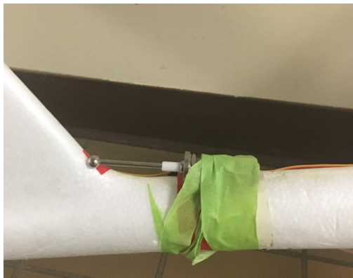
(a) ADS-B antenna in original orientation.
