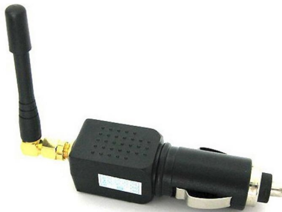
Figure 2.2: Illegal GPS jamming device [6].
