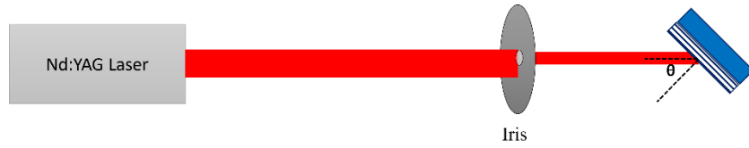
Figure 10. Experimental setup for the nanosecond pulse laser treatment used for processing the Cu/Al multilayer films controlling spot size using mechanical filtering by selectively blocking portions of the beam with an iris aperture.
