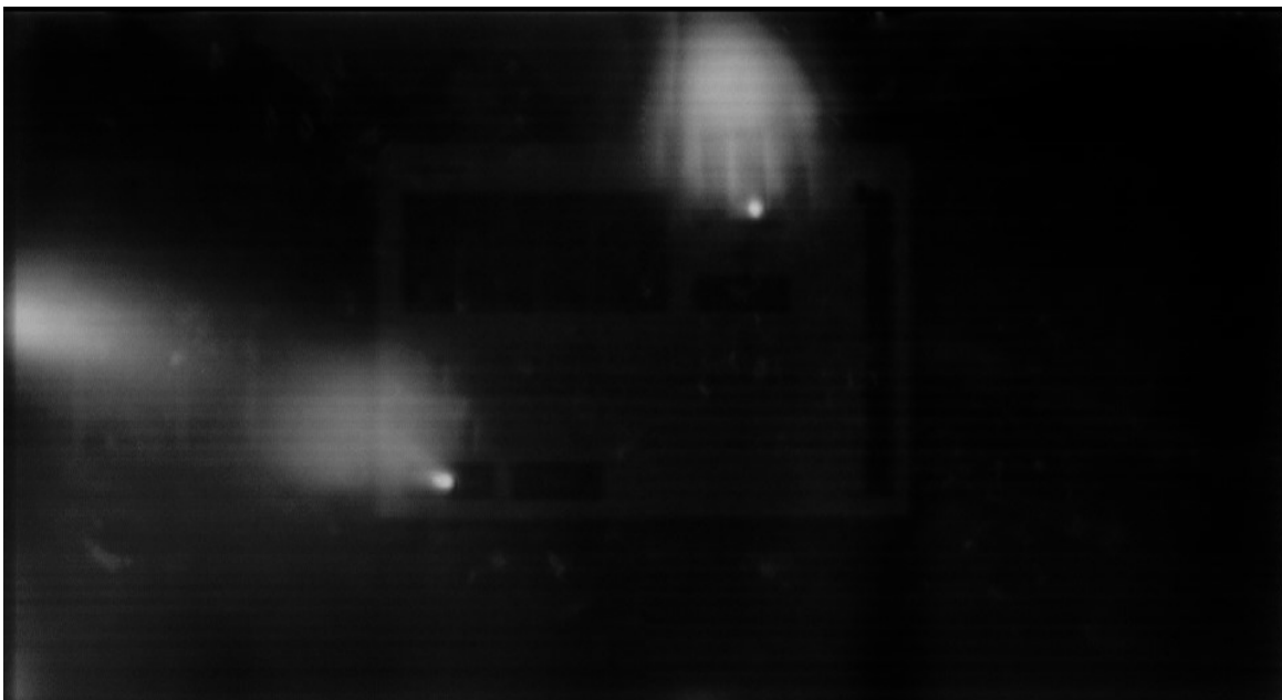
Figure 5-5. A raw image captured by Microsoft PixelSense on board cameras showing two different people touching the screen.
