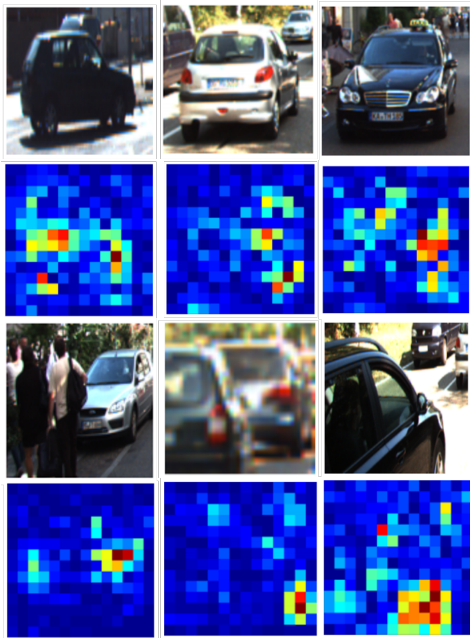
Figure 4.6: Visualization of the learned attention of the model for orientation estimation. The heatmap shows the image areas that contribute to orientation estimation the most. The network attends to certain meaningful parts of the car such as tires, lights, and side mirrors.
