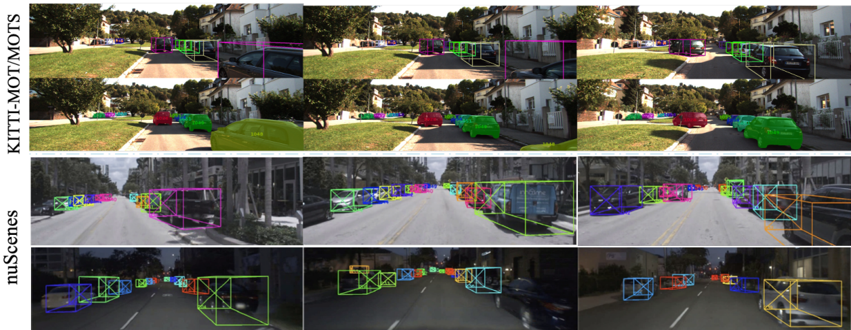
Figure 4.5: Qualitative examples under diverse scenarios. The top row are the results on the KITTI-MOT/MOTS dataset, and the bottom row show the results on some image frames of the nuScenes dataset (daytime and night). The system is capable of estimating the shape and pose (without scale-factor ambiguity) of objects.
