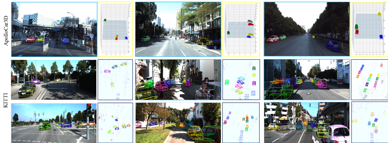
Figure 3.6: Qualitative examples under diverse scenarios. The top row are the results on the ApolloCar3D instances, and the bottom 2 rows show the results on some image frames of the KITTI tracking dataset. The system is capable of estimating the shape and pose (without scale-factor ambiguity) of objects. The images of the scenes contain the projection of the estimated shapes of cars.
