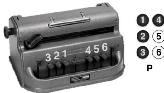
Figure 4. A Perkins Braille on the left and the Braille letter “p” on the right. The numbers above the keys show which keys correspond to which dots in a Braille cell
