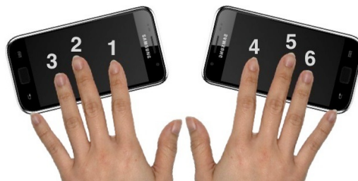
Figure 6. With two devices, the left hand inputs dots 1, 2, and 3 and the right hand inputs dots 4, 5, and 6. The right phone is the primary phone, defined as the phone that initiates the BlueTooth connection and expects dots 4-6 as input.
