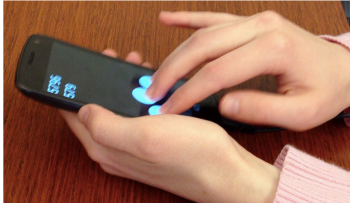
Figure 15. A blind person enters numbers with DigiTaps. The white circles at the bottom of the screen mark her touch points.
