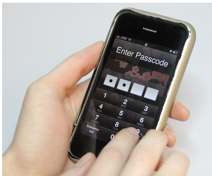
Figure 12. When entering passwords with an iPhone and VoiceOver, a user's input is spoken as she touches the screen, posing a severe security risk.
