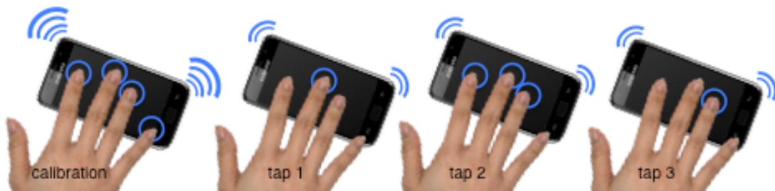
Figure 13. A user calibrates (left) and enters a 3-tap PassChord. The blue circles show which fingers contact the screen in the figure but do not appear as output to the user. Note that the fingers are not striking bounded regions like buttons; rather, the finger locations are interpreted probabilistically, meaning some flexibility in their hit-location is allowed, while the number and identity of the fingers is appropriately strict.
