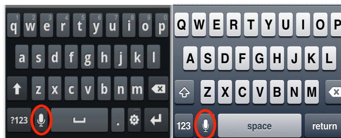
Figure 18. The Android (left) and iPhone (right) keyboards have a dictate button to the left of the space key that enables users to dictate text instead of using the on-screen keyboard.
