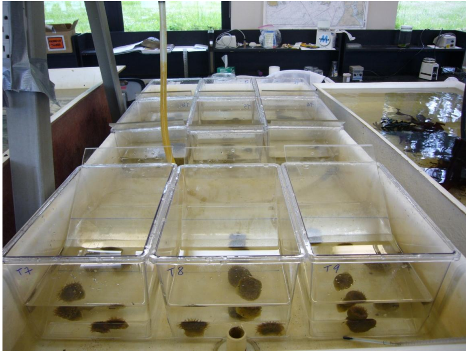
Figure 1. A photo of experimental setup. Nine aquaria submerged in a sea table with running seawater to keep the temperature constant.
