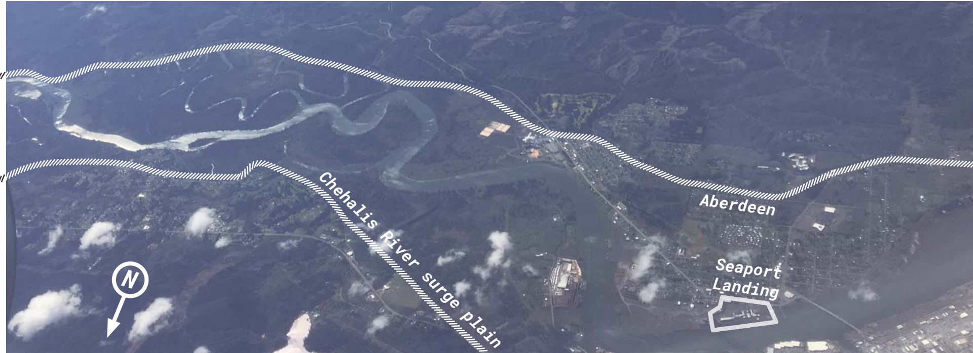
Fig. 2-8. Tracing the edges of the estuary's floodplain highlights overlaps between the historic Chehalis River surge plain and developed lowlands of Aberdeen. (photo: Anna Tamura, National Parks Service)
