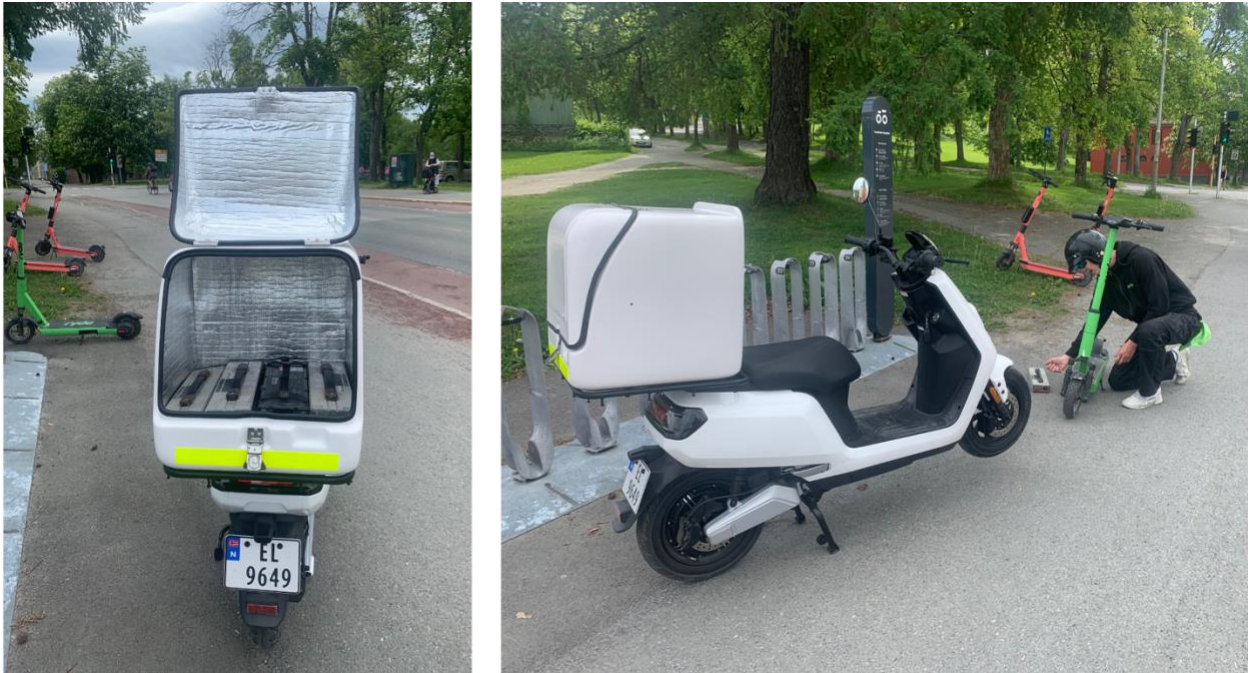
Figure 2.5. Battery servicing by Ryde in Trondheim, Norway. The electric service scooter can safely transport up to 8 kick scooter batteries in its cargo box. The service technician field swaps the batteries in approximately one minute.
