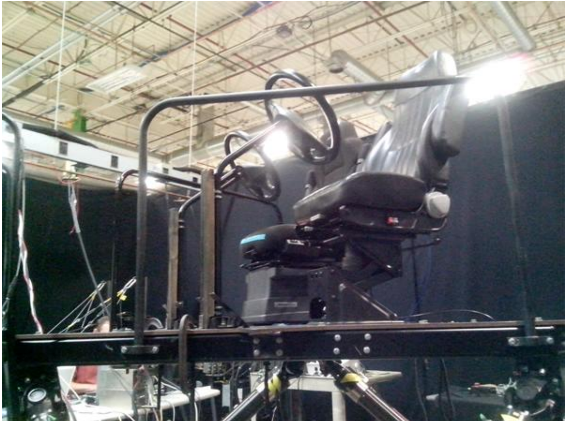
Figure 5: Hexapod mounted with the two truck seat seats, the active suspension seat is in the background and the passive suspension seat in the foreground.
