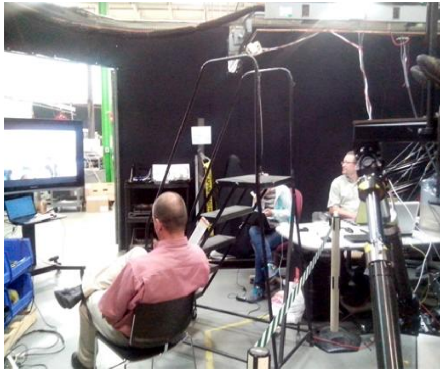
Figure 6: Experimental set-up showing the large screen TV the subjects were supposed to watch while sitting on the hexapod
