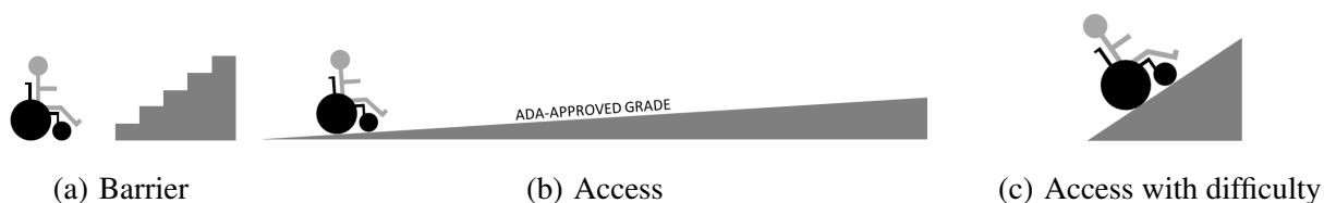
Figure 6.2: Three images of a wheelchair user provide visual metaphors of disability barriers and access issues: (a) Stairs are an absolute barrier to access. (b) A ramp with an ADA-compliant grade (to scale) provides access. (c) A ramp with a larger grade allows access, but with difficulty.
