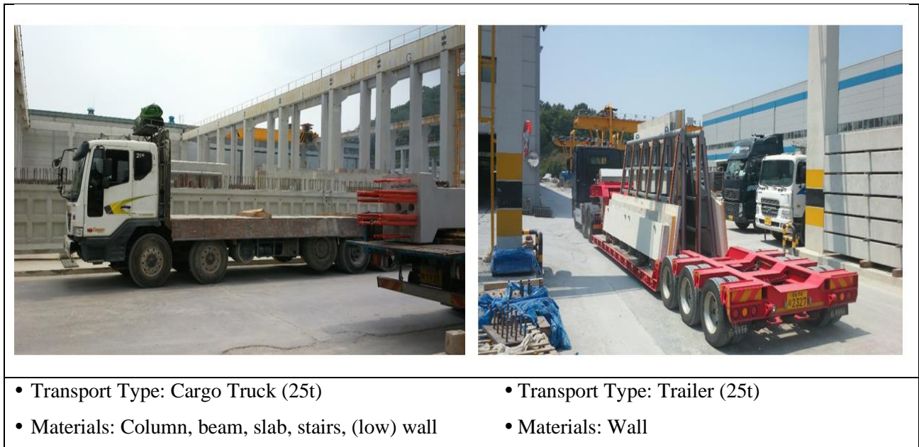
Figure 18. Transportation Type for Panelized Module of Case Study
