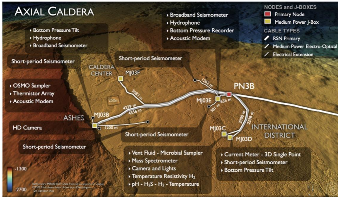
Figure 2. The Axial Caldera and instruments present. The presence of short-period and broadband seismometers are the most important instruments in registering earthquakes to send back through the cabled array (Reproduced from Kelley et al., 2014).
