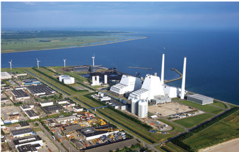
Figure 2-12. The industrial zone in Kalundborg, Denmark, is designed to share and recycle energy and resources among disparate production types and complexes.
