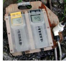
There is a place on the holder for both a conductivity meter and the DO meter.
