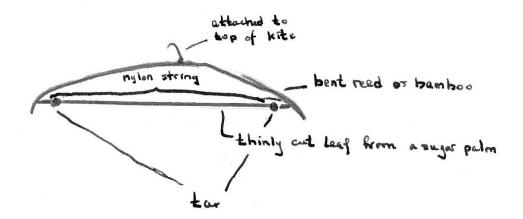
If this instrument is moved rapidly through the wind, the palm leaf will make a deep vibrating sound. Thus when it is placed on top of the kite, the wind and motion of flying the kite will cause it to vibrate.
