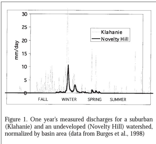
Figure 1. One year's measured discharges for a suburban (Klahanie) and an undeveloped (Novelty Hill) watershed, normalized by basin area (data from Burges et al., 1998)
