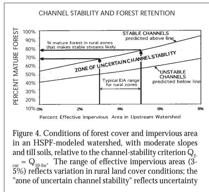
Figure 4. Conditions of forest cover and impervious area in an HSPF-modeled watershed, with moderate slopes and till soils, relative to the channel-stability criterion  $Q_{2-cur} = Q_{10-for}$ . The range of effective impervious areas (3-5%) reflects variation in rural land cover conditions; the "zone of uncertain channel stability" reflects uncertainty
