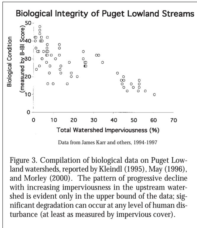
Figure 3. Compilation of biological data on Puget Lowland watersheds, reported by Kleindl (1995), May (1996), and Morley (2000). The pattern of progressive decline with increasing imperviousness in the upstream watershed is evident only in the upper bound of the data; significant degradation can occur at any level of human disturbance (at least as measured by impervious cover).
