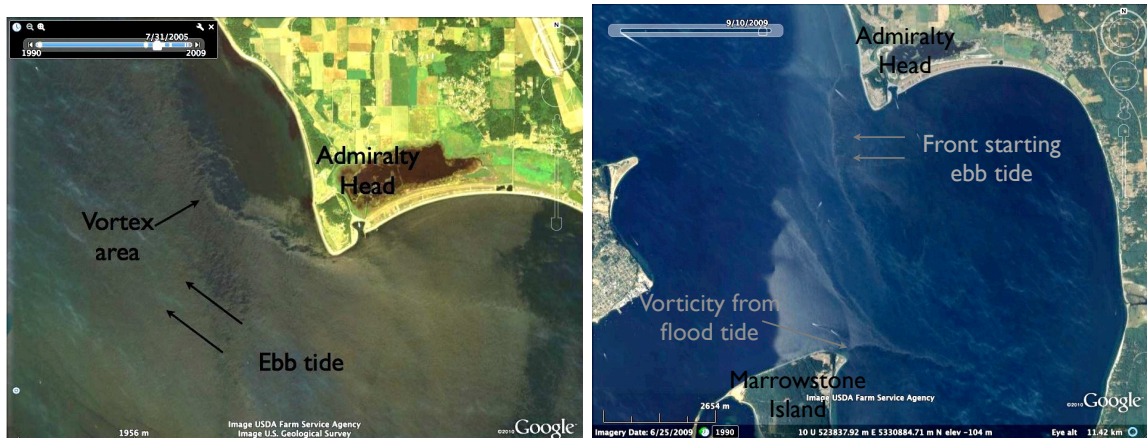
(a) The surface disruption due to a headland-generated eddy streaming off Admiralty Head on ebb changes from flood to ebb, near Admiralty Head. (b) A front moves through the system as the tide. Near the northeast corner of Marrowstone Island, vorticity from flood tide is still visible.
