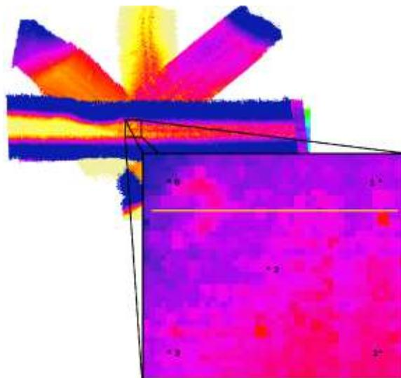
*Figure 4. ArcGIS 10.1, image of the transect compilation, with a magnified projection of the Analysis Region (AR). In the AR five points have been selected to for evaluation of depth estimates variance over time, as well as a pixel segment that has been selected for evaluation of depth estimate variance over a distance at various time intervals (yellow line).*
