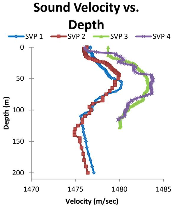
Figure 5. Sound velocity profiles of the first four transects, illustrating changes in sound velocity during the 7.5 hour survey. Not shown is the baseline standard of  $1500 \text{ m s}^{-1}$ , which is a straight line down ward from 1500 m.
