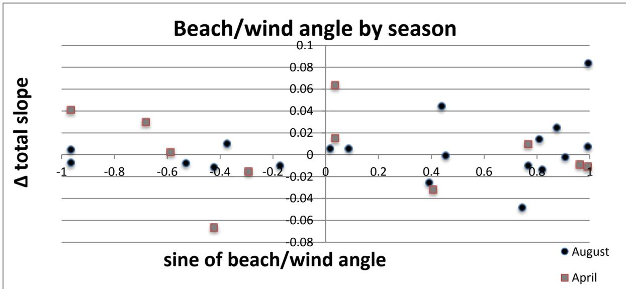
Figure 7 Study beaches divided into April and August groups by the date profile was taken. Negative sine values indicate offshore wind conditions, positive sine values indicate onshore wind conditions. Positive total slope values indicate steeper armored beaches and negative values are steeper unarmored beaches. Sine values of 1 indicate orthogonal winds and of 0 indicate parallel winds to beach.
