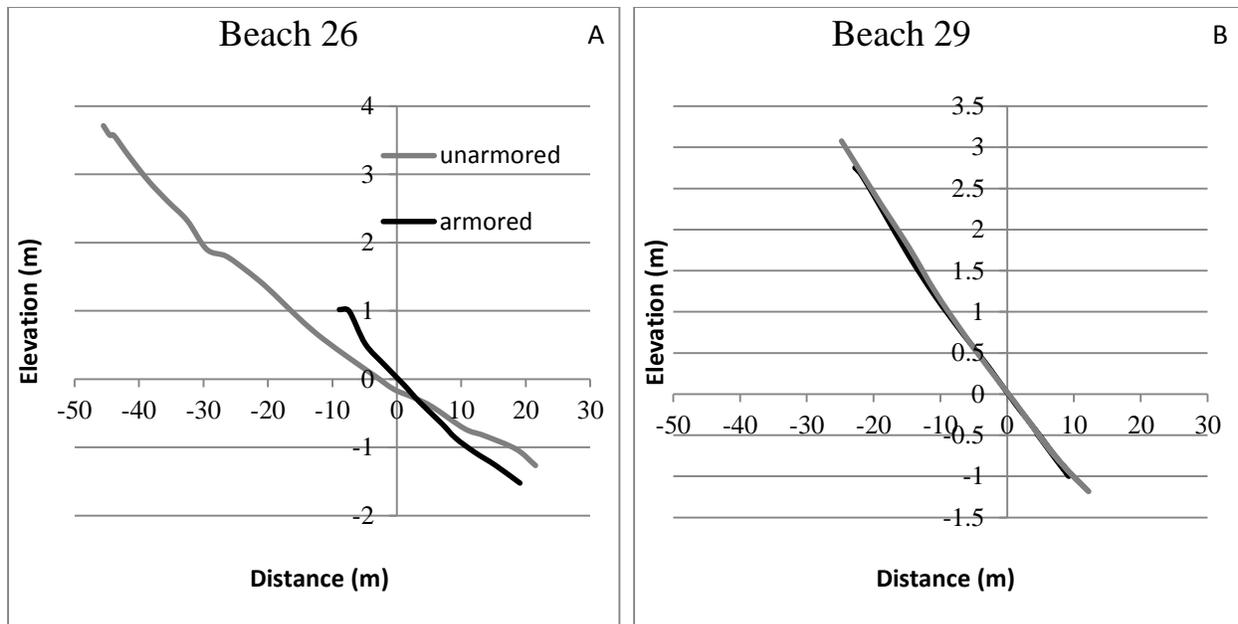
Figure 8 Profiles of Beaches #29 (Anderson Island) and #26 (McNeil Island) showing elevation and horizontal distances between MLW and top of berm or toe of seawall.
