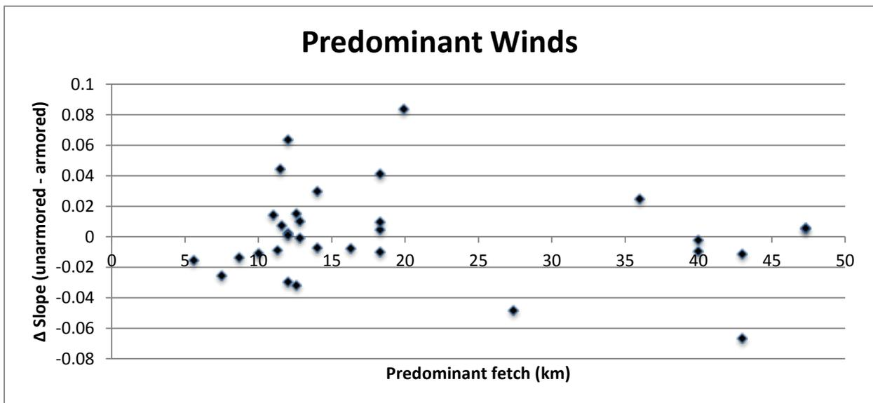
Figure 5 *Predominant wind regime, in kilometers of fetch, compared to change in slope between armored and unarmored sections of 31 pairs of beaches. Predominant fetch is the direction of the longest possible onshore fetch for each pair of beaches. The change in slope is positive for steeper armored beaches, and negative for steeper unarmored beaches within each pair.*
