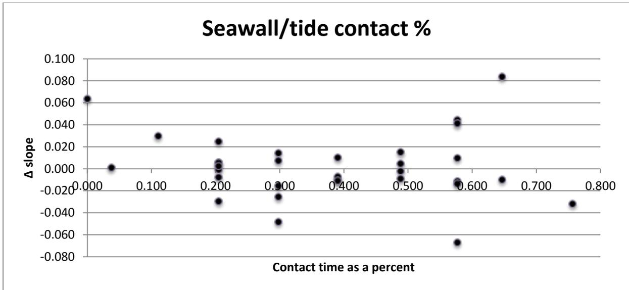
Figure 6 Changes in slope relative to the percent time the tide is in contact with a seawall. A lower contact percentage indicates a seawall higher on the beach face.
