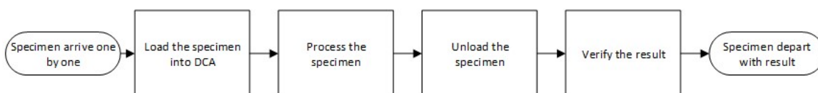
Figure B.1: Flowchart of analytical process on a DCA instrument.
