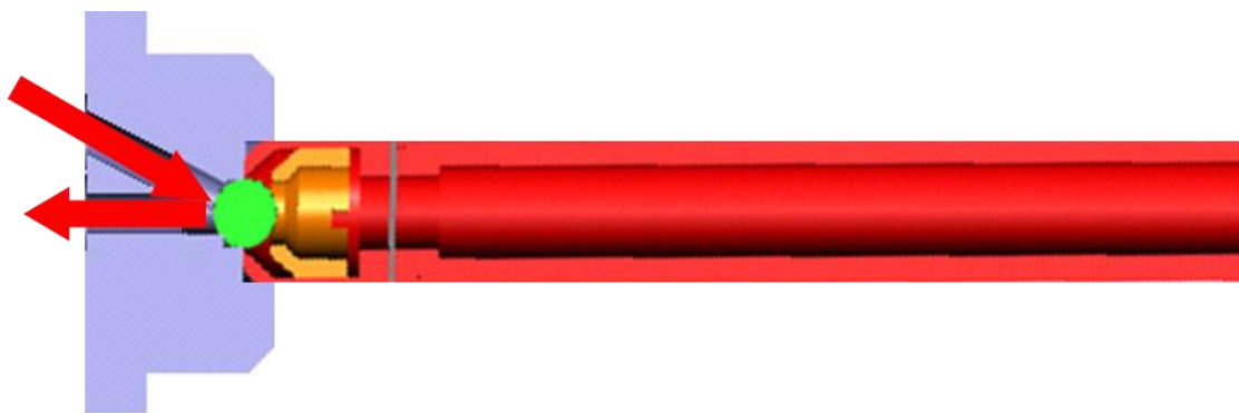
Figure 1.8. A schematic of a Raman BallProbe™ interfaced with the flow channel of a NeSSI sampling piece.
