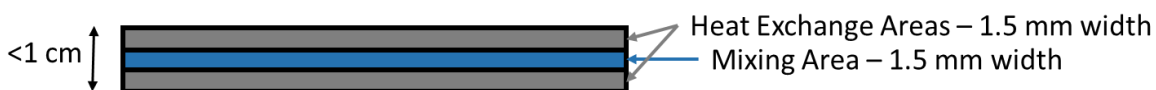
Figure 1.1. Schematic side-view of continuous flow reactor mixing chip showing heat exchange and mixing areas. Each layer has a width of 1.5 mm, and is separated by 1 mm of glass.
