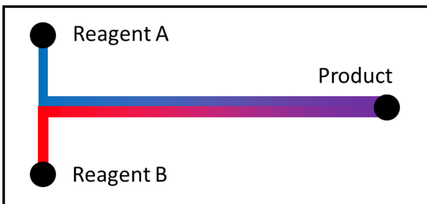
Figure 1.2. T-junction micromixer schematic. Two reagents (red and blue) mix slowly via diffusion on the path towards the reactor exit.
