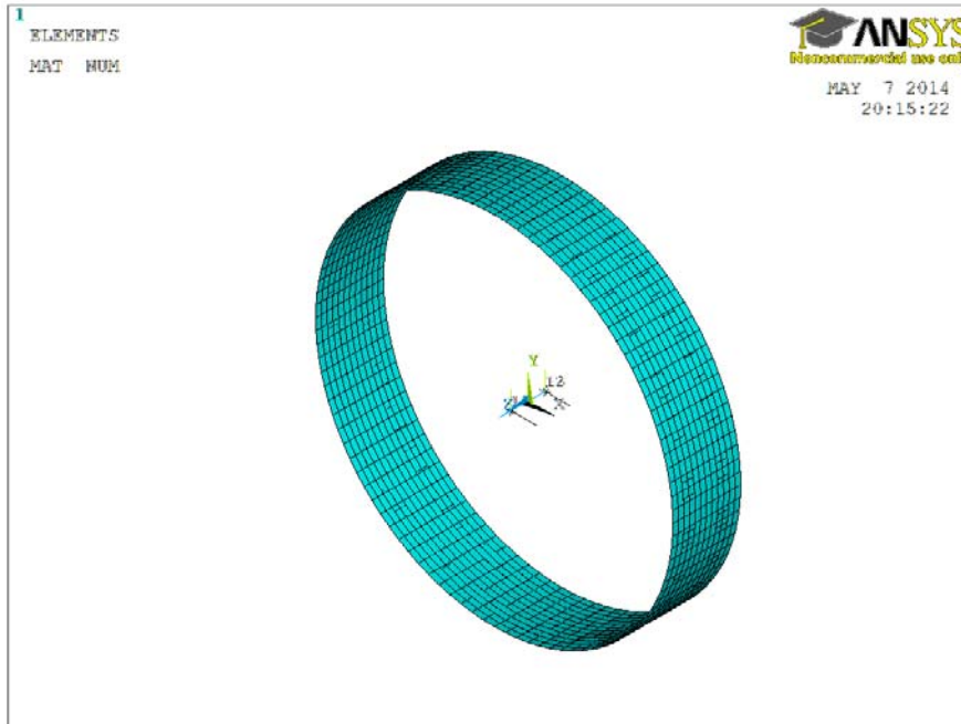
Figure 3: The Bearing. The Contact Element CONTA174 Constrains the DOF of the Inner and Outer Races to the Pilot Nodes Created by the Target Element Which is Later Connected to MPC184 General Joints via MPC184 Rigid Beam. The Two Local Coordinates Indicate the Position of the Pilot Nodes. The Stiffness is Defined as Material Property of the Joints.
