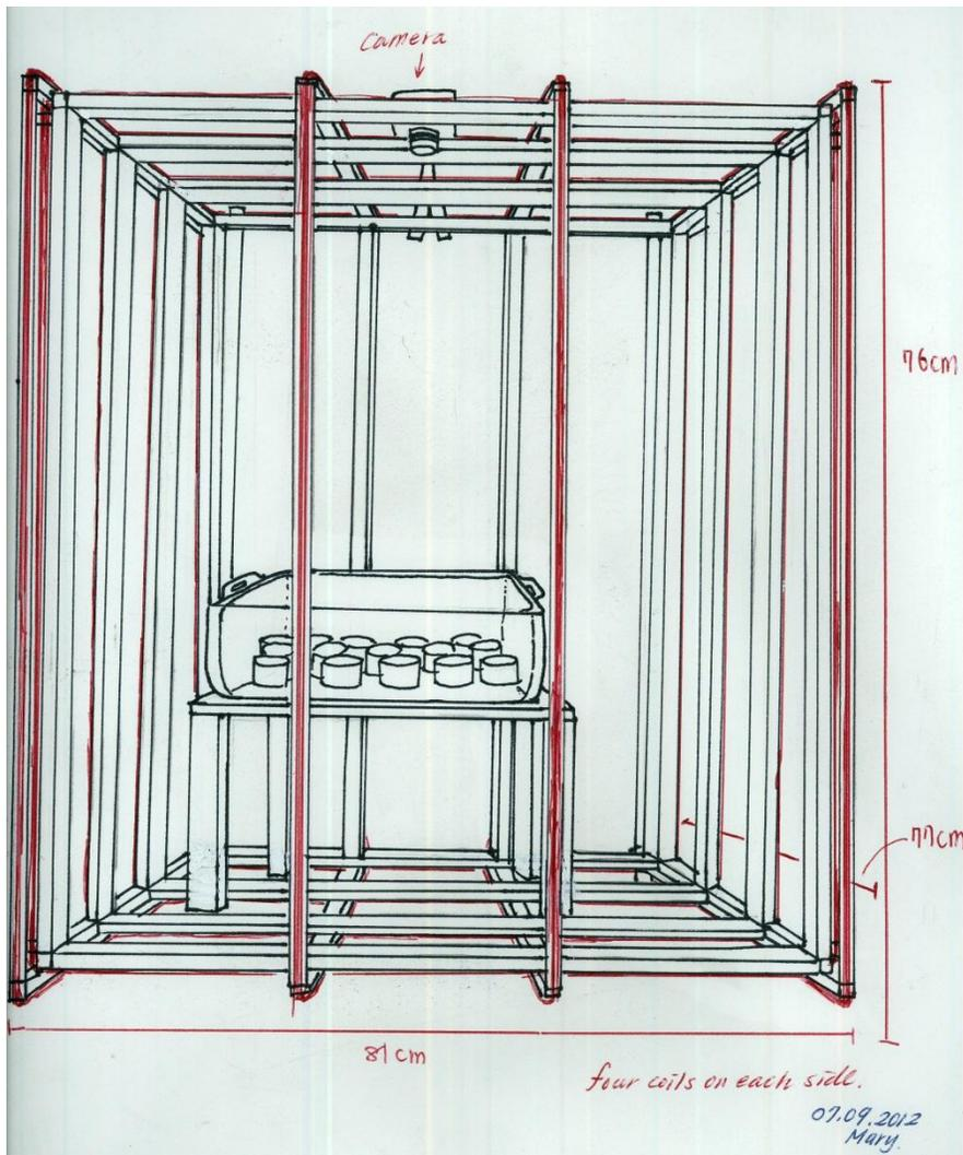
Fig. 1. Magnetic stimulus was generated by a magnetic coil system (4 square coils, each 1.02m on a side). Constant current was introduced and flowed through the circular wire. This created a magnetic field around the coiled wire magnetizing the metal as if it were a permanent magnet. Organisms were exposed to a magnetic field intensity of 100,000 nT which is the same intensity of ambient field.
