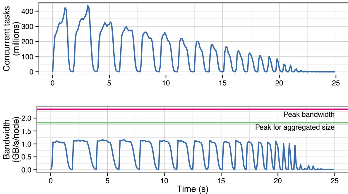
Figure 4.5: Grappa PageRank execution over time on 32 nodes. The top shows the total number of concurrent tasks (including delegate operations), over the 85 iterations, peaks diminishing as fewer vertices are being updated. The bottom shows message bandwidth per node, which correlates directly with the concurrency at each time step, compared against the peak bandwidth, and the bandwidth for the given message size.
