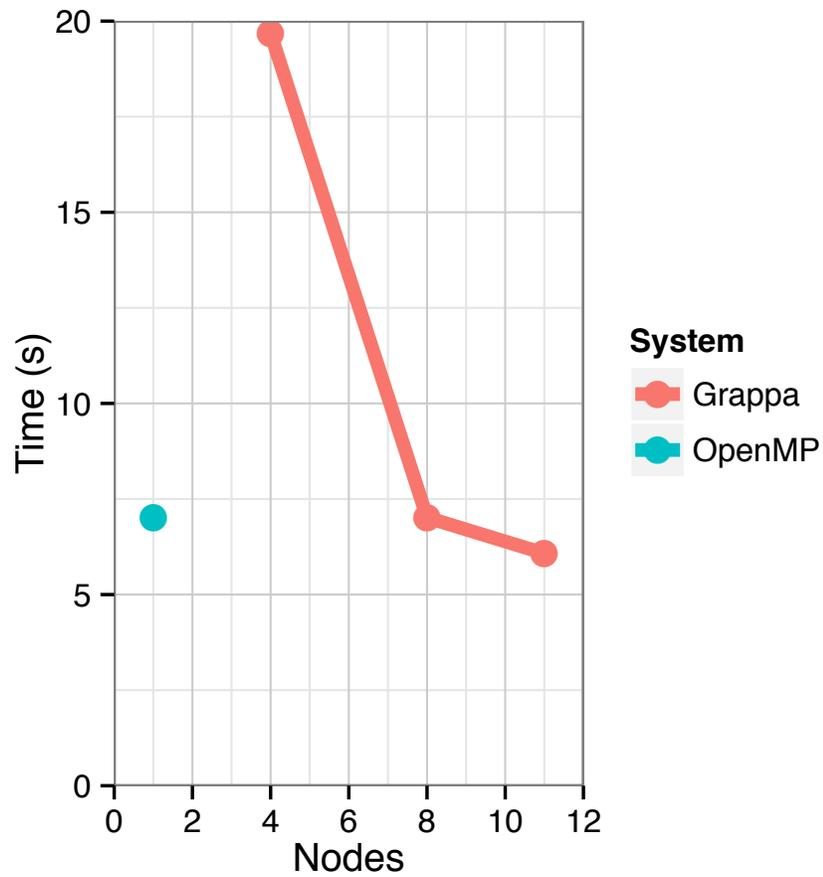
Figure 4.15: Performance of BFS on one node using OpenMP compared to multiple nodes using Grappa with 8 cores per node. On 8 nodes, Grappa matches the performance of the OpenMP version; with more nodes Grappa exceeds OpenMP's performance.
