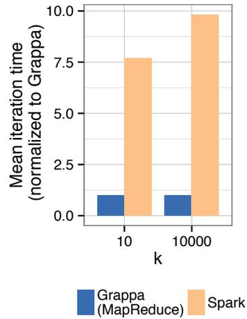
Figure 4.8: Data parallel experiments using k-means on a 8.9GB Seaflow dataset running on 64 nodes. Grappa’s performance advantage comes primarily from its network layer as well as reduced iteration overhead as in the Shark comparison (Figure 4.7).
