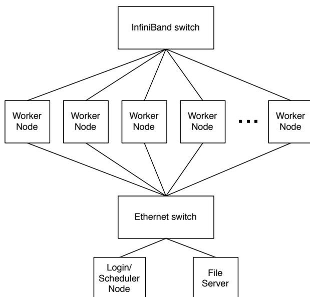
Figure 2.1: Schematic of cluster used for limit experiments.
