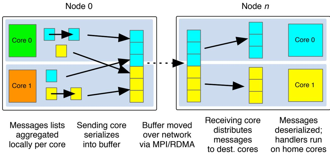
Figure 3.4: Message aggregation process.
