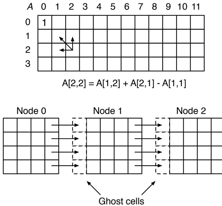
Figure 4.13: Structure of Intel stencil kernel. The top figure shows the logical view of the computation of one cell. The bottom figure shows how the benchmark is mapped to the cluster; ghost cells are denoted with dotted lines, and arrows show how values are communicated between nodes.
