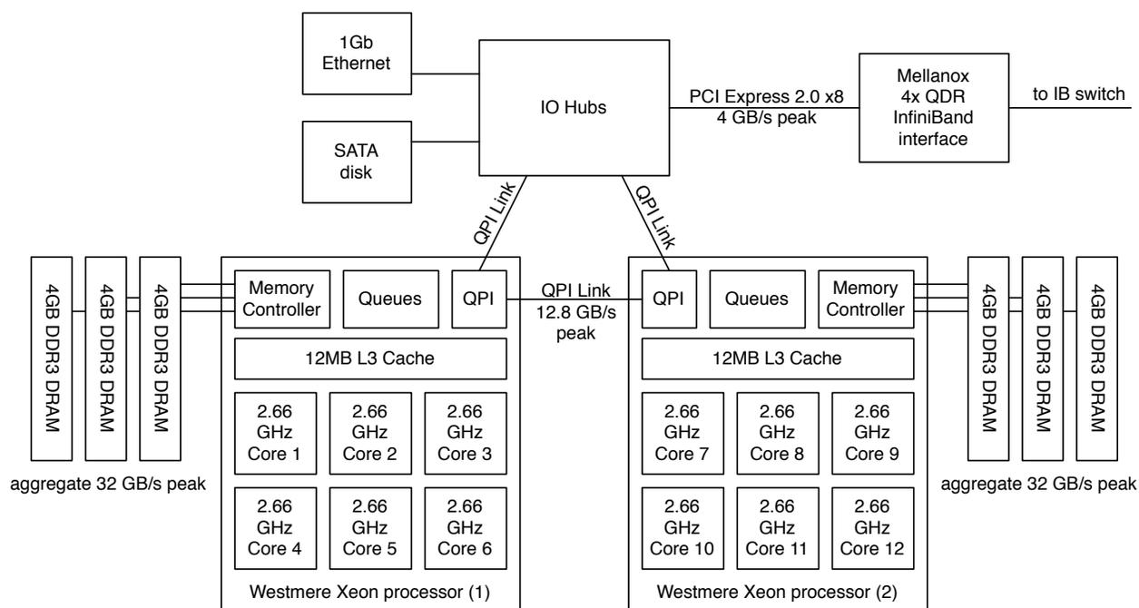
Figure 2.2: Schematic of cluster node used for limit experiments.
