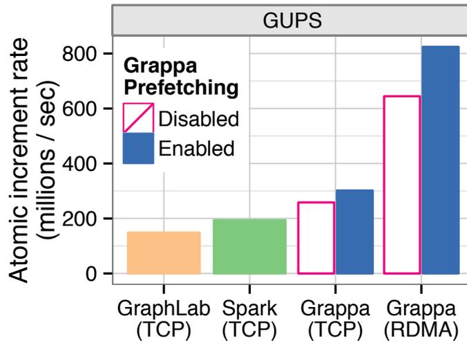
Figure 4.4: GUPS message rates for GraphLab, Spark, and Grappa on 31 nodes. Grappa is shown using both TCP-based and RDMA-based configuration, with message prefetching on and off.
