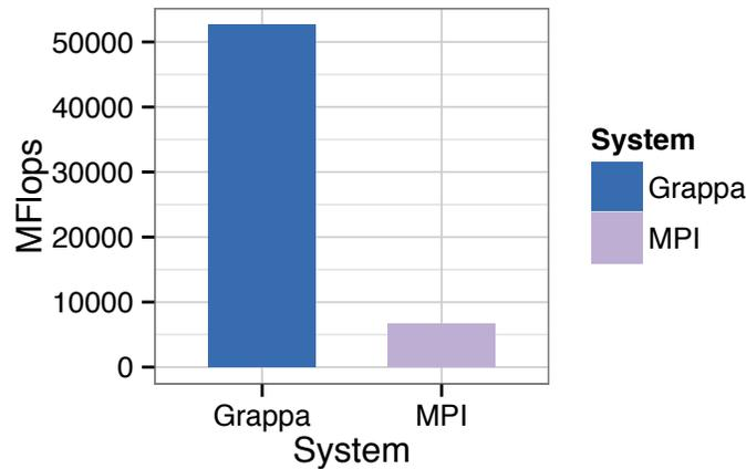
Figure 4.14: Performance of Intel stencil kernel on Grappa compared with reference MPI version on 8 nodes with 8 cores per node. Grappa is able to aggregate updates to ghost cells which increases the amount of pipeline parallelism and thus performance.
