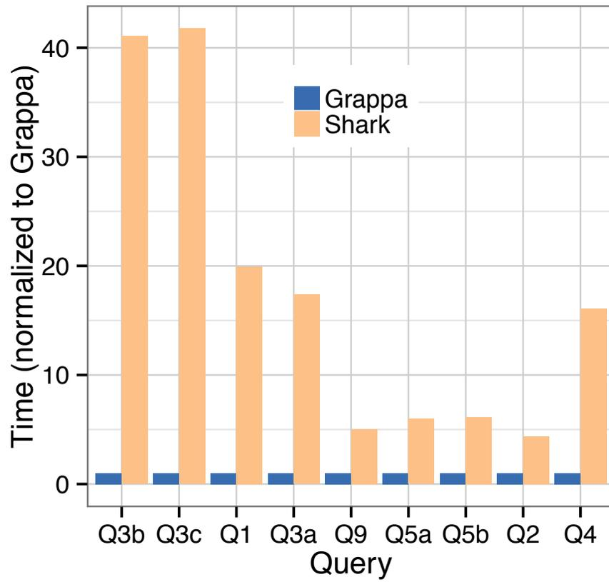
Figure 4.6: The SP<sup>2</sup>Bench benchmark on 16 nodes. Query Q4 is a large workload so it was run with 64 nodes.
