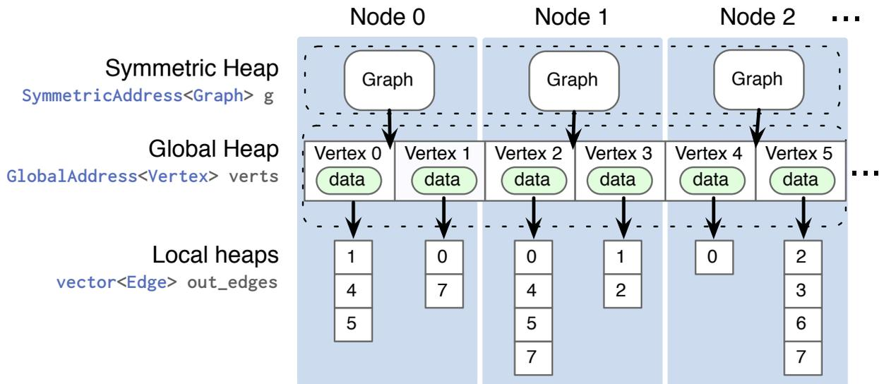
Figure 3.2: Using global addressing for graph layout.
