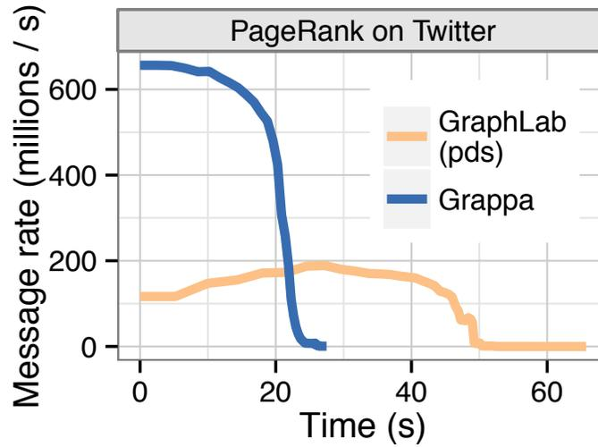
Figure 4.3: Cluster-wide message rates (average per iteration) while computing PageRank on 31 nodes, comparing Grappa with GraphLab using their PDS partitioning strategy.
