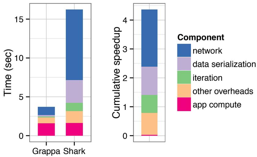
Figure 4.7: Performance breakdown of speedup of Grappa over Shark on Q2. Both systems spend the same time doing computation; Grappa’s increased performance comes primarily from its more efficient use of the network, with an additional benefit from its use of compiled queries, which show up as iteration and serialization time for Shark.
