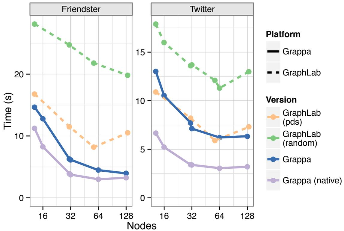
Figure 4.10: Scaling BFS out to 128 nodes. In addition to Grappa’s vertex-centric engine, we also show a custom algorithm for BFS implemented natively which employs Beamer’s bottom-up optimization to achieve even better performance.
