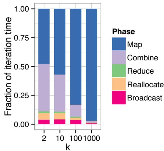
Figure 4.9: Breakdown of time spent in MapReduce phases for Grappa-MapReduce for k-means on the Seaflow dataset.
