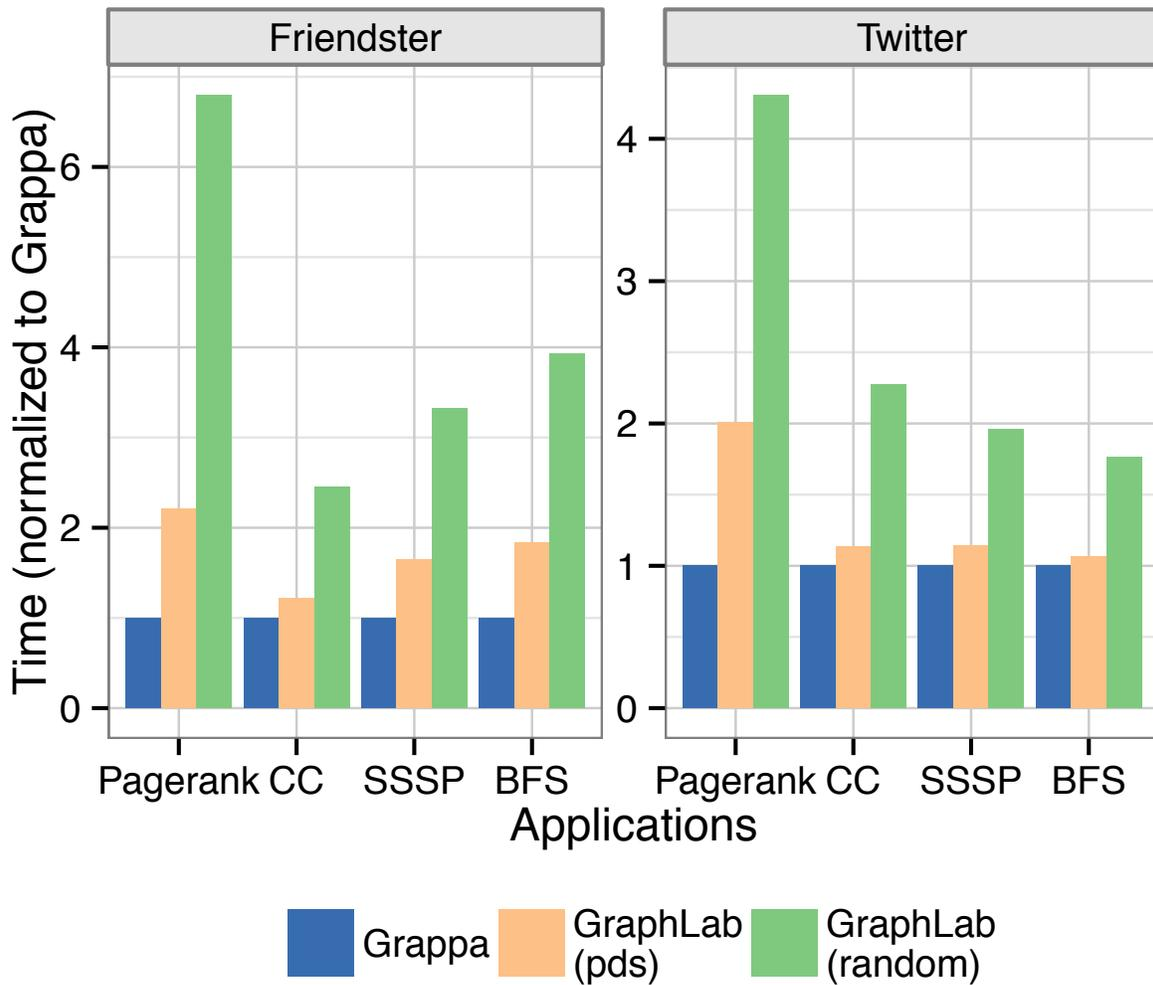
Figure 4.1: Vertex-centric performance of Grappa compared to GraphLab with random and with optimized PDS partitioning strategies, showing time to converge (same number of iterations) normalized to Grappa, on the Twitter and Friendster datasets, running on 31 nodes.
