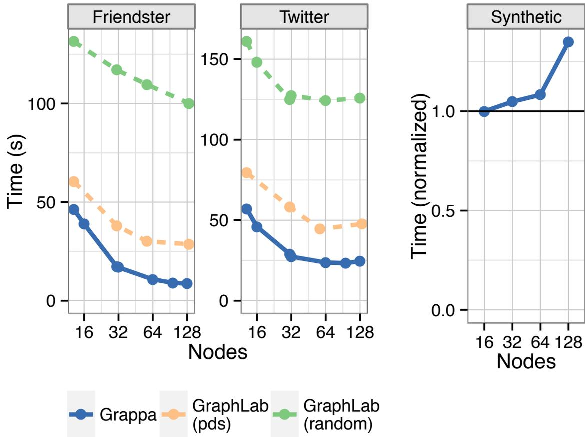
Figure 4.2: Vertex-centric scaling results for PageRank out to 128 nodes. On the left we use the Friendster and Twitter datasets to measure *strong* scaling, which is limited in this case by the size of the datasets. We compare Grappa with GraphLab using both their random and optimized PDS partitioning strategies. On the right we use synthetic power-law graphs scaled proportionally with cluster node count to measure *weak* scaling.
