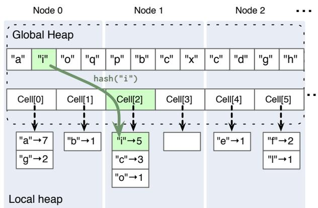
Figure 1.1: “Character count” with a simple hash table implemented using Grappa’s distributed shared memory.
