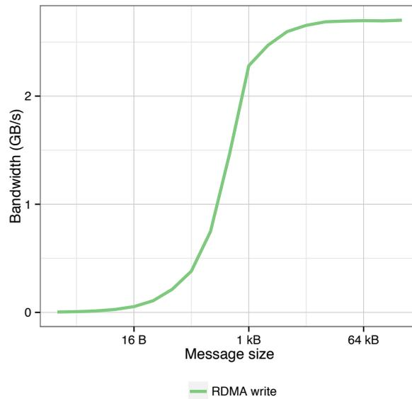
Figure 2.5: RDMA write performance between two cluster nodes. For small messages, only a fraction of the network bandwidth is able to be used.
