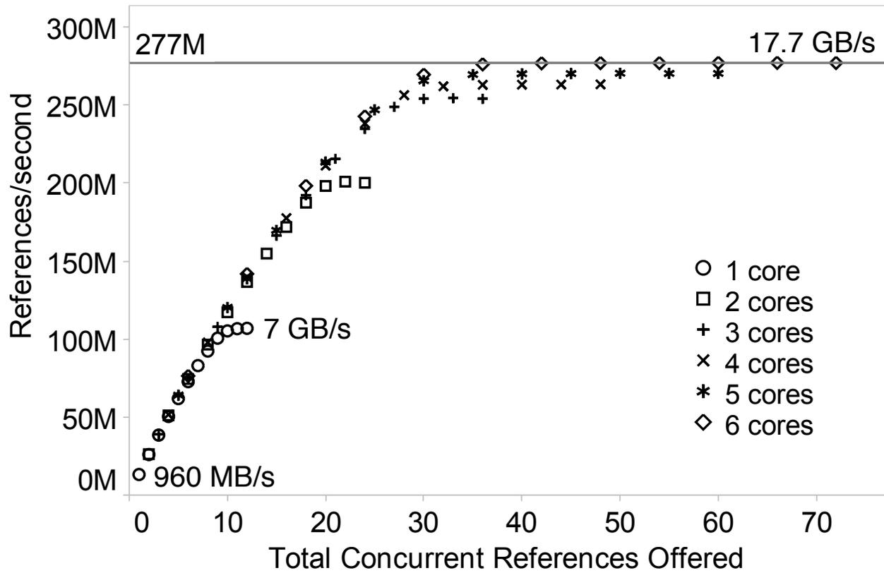
Figure 2.4: Random access to socket-local memory with varying number of concurrent references per core.
