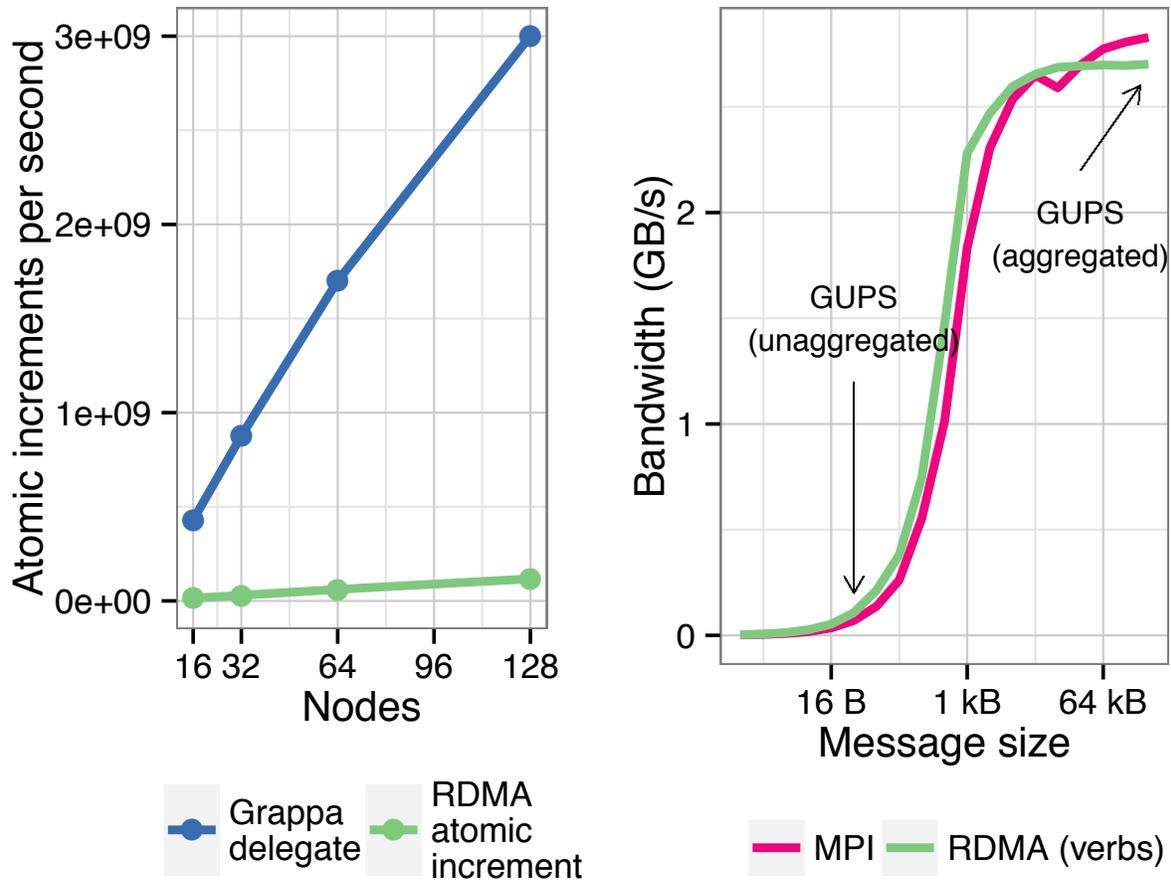
Figure 3.5: On the left, random updates to a billion-integer distributed array with the GUPS benchmark. On the right, ping-pong bandwidth measured between two nodes.
