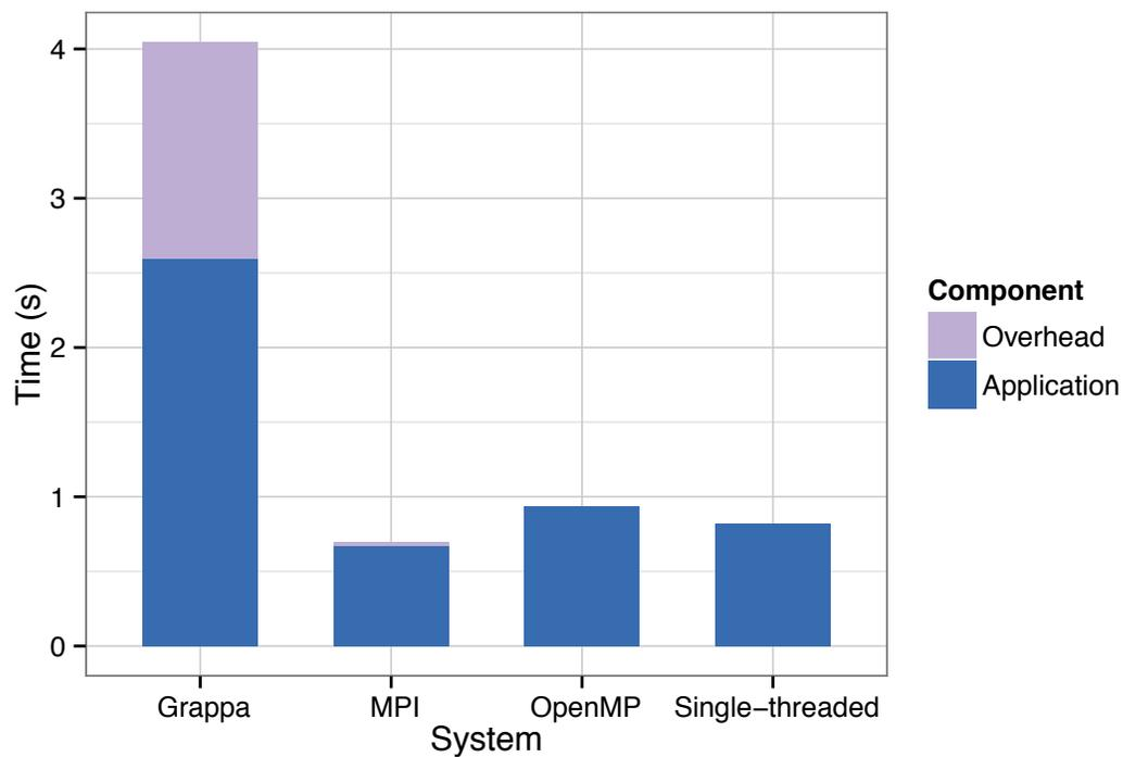
Figure 4.11: Single-core performance of BFS on Grappa compared with three implementations from the Graph500 benchmark. *Overhead* represents time spent converting global addresses to local addresses, expanding the recursive loop decomposition, and calling functions in the MPI library, even though no communication is occurring. *Application* time is spent inspecting and updating vertices.
