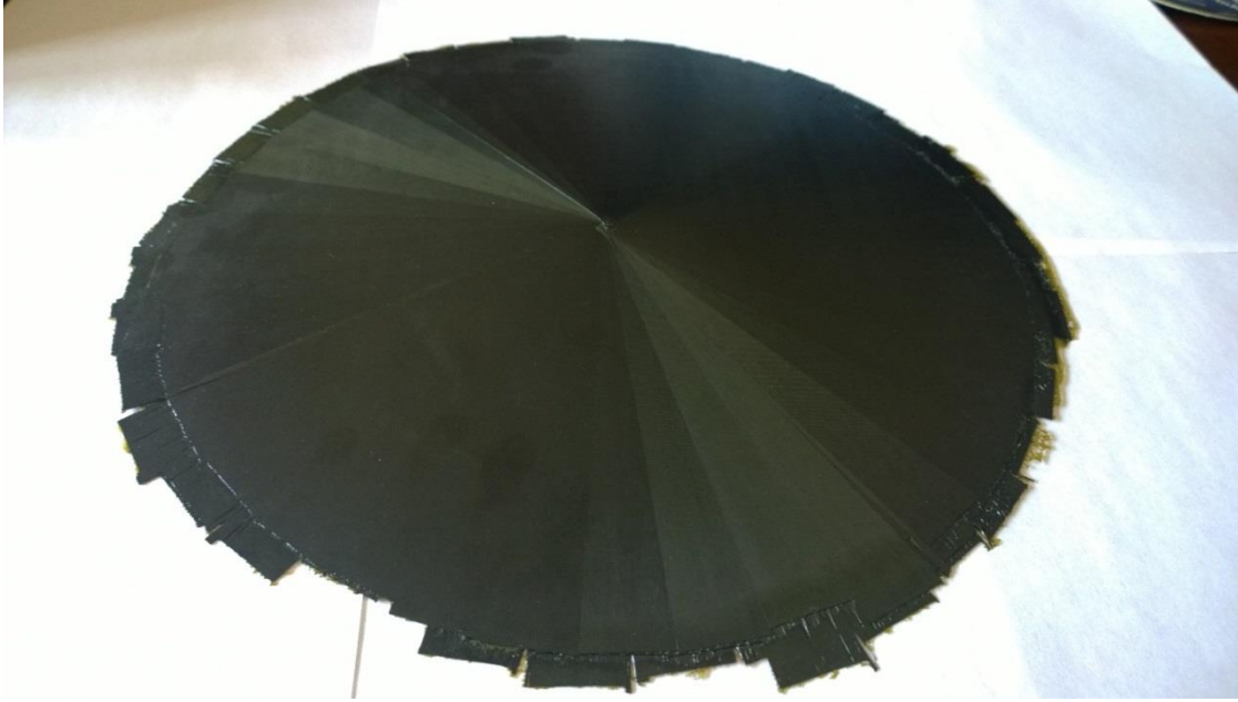
FIGURE 2: SHALLOW CONICAL SHAPE OF ONE-POLE PANEL AFTER CURE
