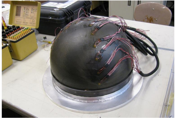
FIGURE 26: STRAIN GAUGE ROSETTE AND DOME WITH STRAIN GAUGES MOUNTED
