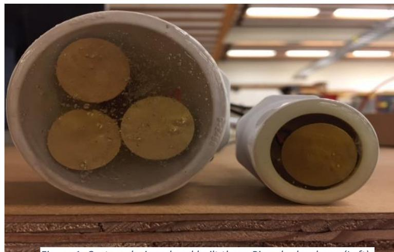
*Figure 1. Custom designed and built three-Piezo hydrophone (Left) and one-Piezo hydrophone housed in PVC, potted in epoxy.*
