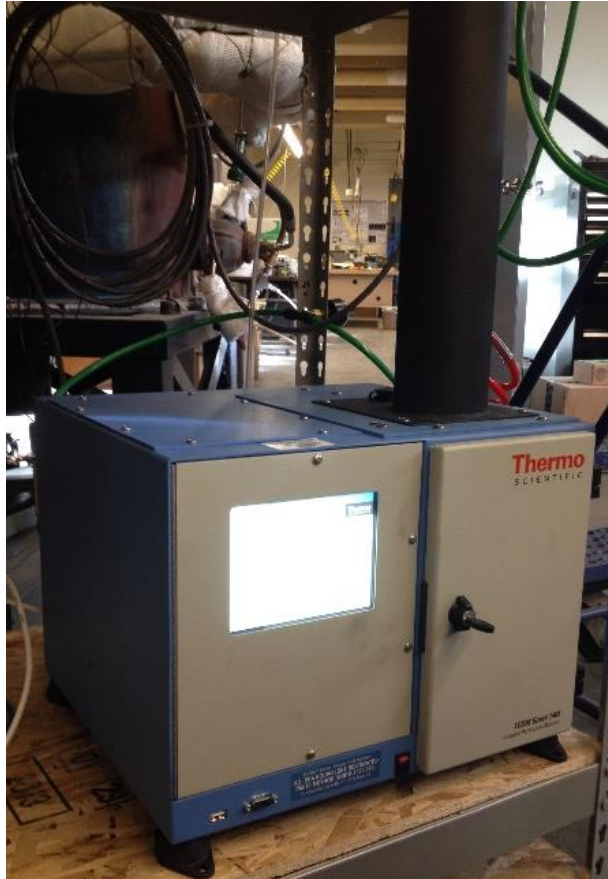
Figure 4: ThermoScientific TEOM 1405 system. The oscillating filter assembly is located in the lockbox on the right. The data output screen and interface is located to the left.
