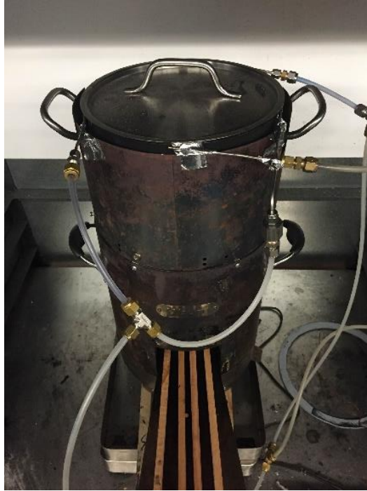
Figure 23: Experimental setup for measuring excess air within a natural draft cookstove. Four 3/16" OD stainless steel sampling probes are positioned and taped in a diamond configuration at the top of the pot skirt, so that they sample the combustion gases in the gap between the pot and the pot skirt. These sample lines then converge to a single sample line which is connected to a CO 2 analyzer.
