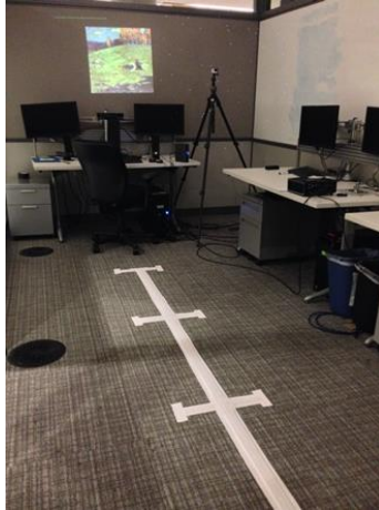
Figure 6.2. Eyes-Free Art presented in a room. The painting is projected on the wall to simulate a gallery, with the Kinect sensor below. On the floor is a white tape and cardboard “ladder” used as a tactile cue to navigate between the 4 zones.
