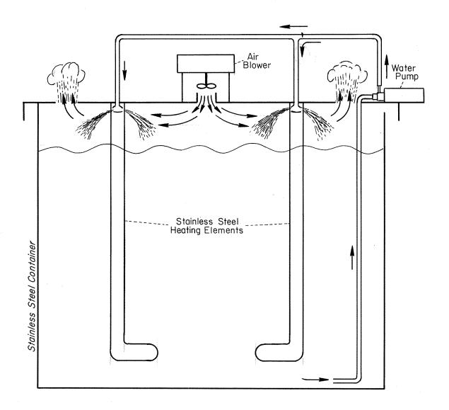
Fig. 2. Stainless steel concentrator used in simulating blowdown water.
