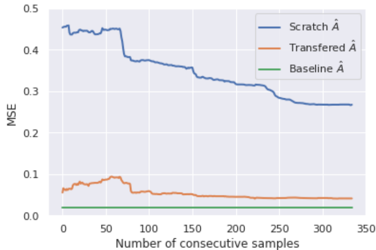
Figure 4.3: Validation MSE of SEB’s \hat{A}_2 state transition matrix learned with an increasing number of consecutive hourly samples (normalized in 0-1 over training data) with (“transfer”) and without (“scratch”) including data from EnergyPlus simulations of building 1
