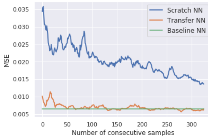
Figure 4.4: Validation MSE of SEB’s \mathbf{F}_2 neural network learned with an increasing number of consecutive hourly samples (normalized in 0-1 over training data) with (“transfer”) and without (“scratch”) including data from EnergyPlus simulations of building 1
