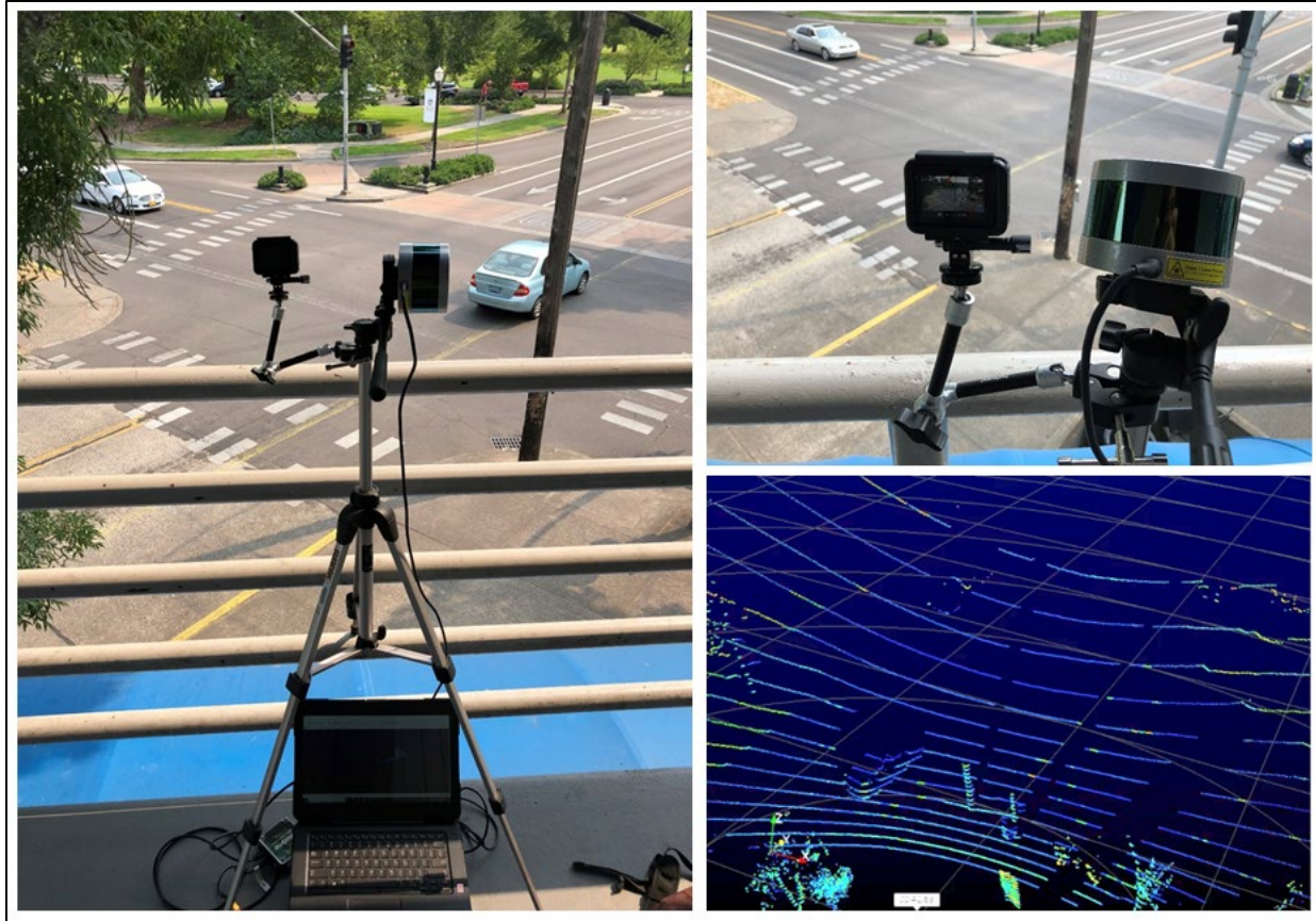
Figure 3.4 Stationary lidar data acquisition overlooking intersection.
