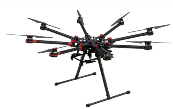
Figure 2.2.1 DJI S1000 airframe selected for this project.
