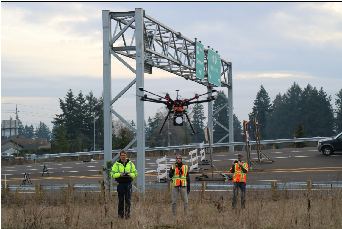
Figure 3.1 UAS data collection at the Newberg Dundee construction site.
