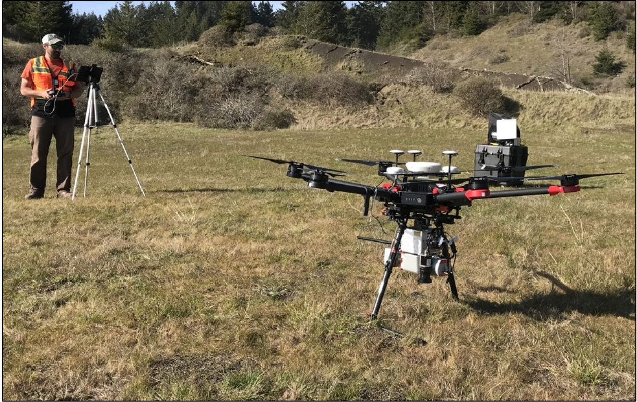
Figure 3.5 Phoenix Lidar Systems MiniRanger, incorporating a Riegl miniVUX-1UAV lidar.
