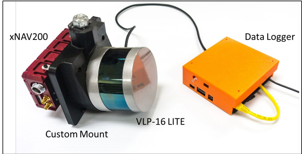
Figure 2.2.3 Final sensor payload including xNAV200 rigidly fixed to the custom mount (left) and the data-logger for the VLP-16 LITE (right).
