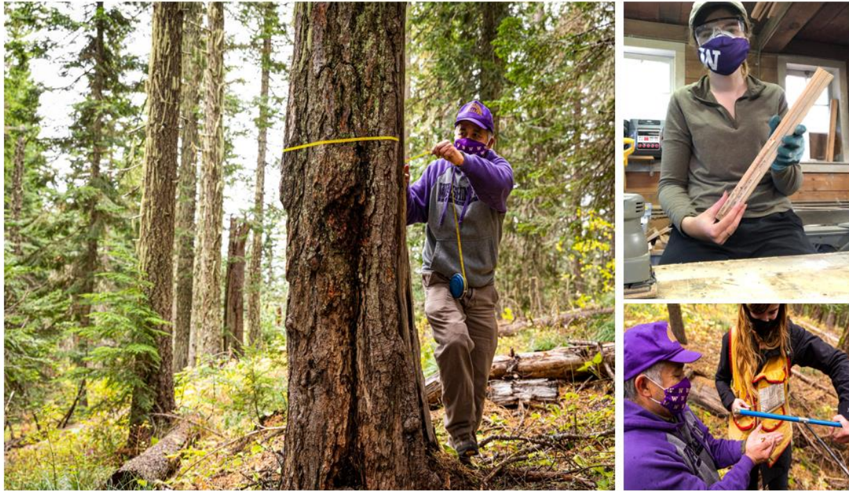
Figure 7. Images illustrating the tree coring process by taking initial measurements of the tree of interest which was a western larch in this case, using a Haglof increment borer to collect the core, and finally sanding the mounted and labeled core at Pack Forest in Eatonville, Washington. Photo Credit: Mark Stone.
