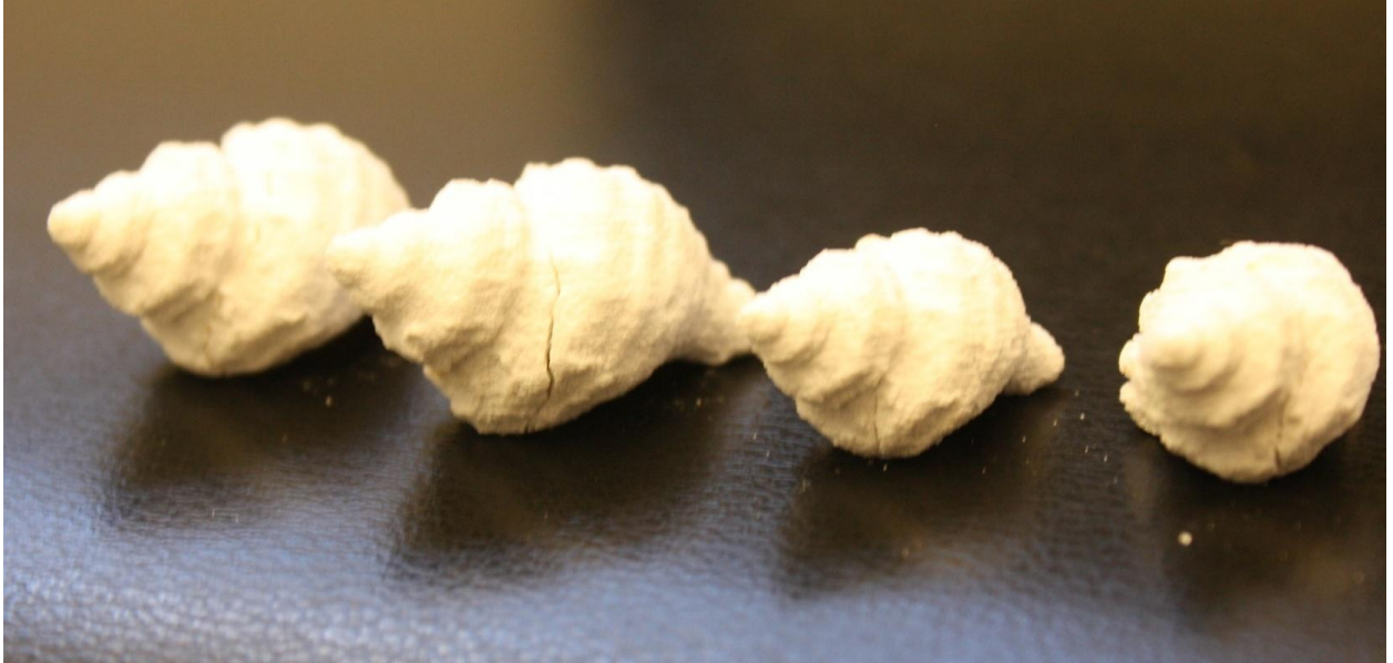
Figure 7: Photo of consistent structural failure patterns (crack propagation) in prototyped shells.
